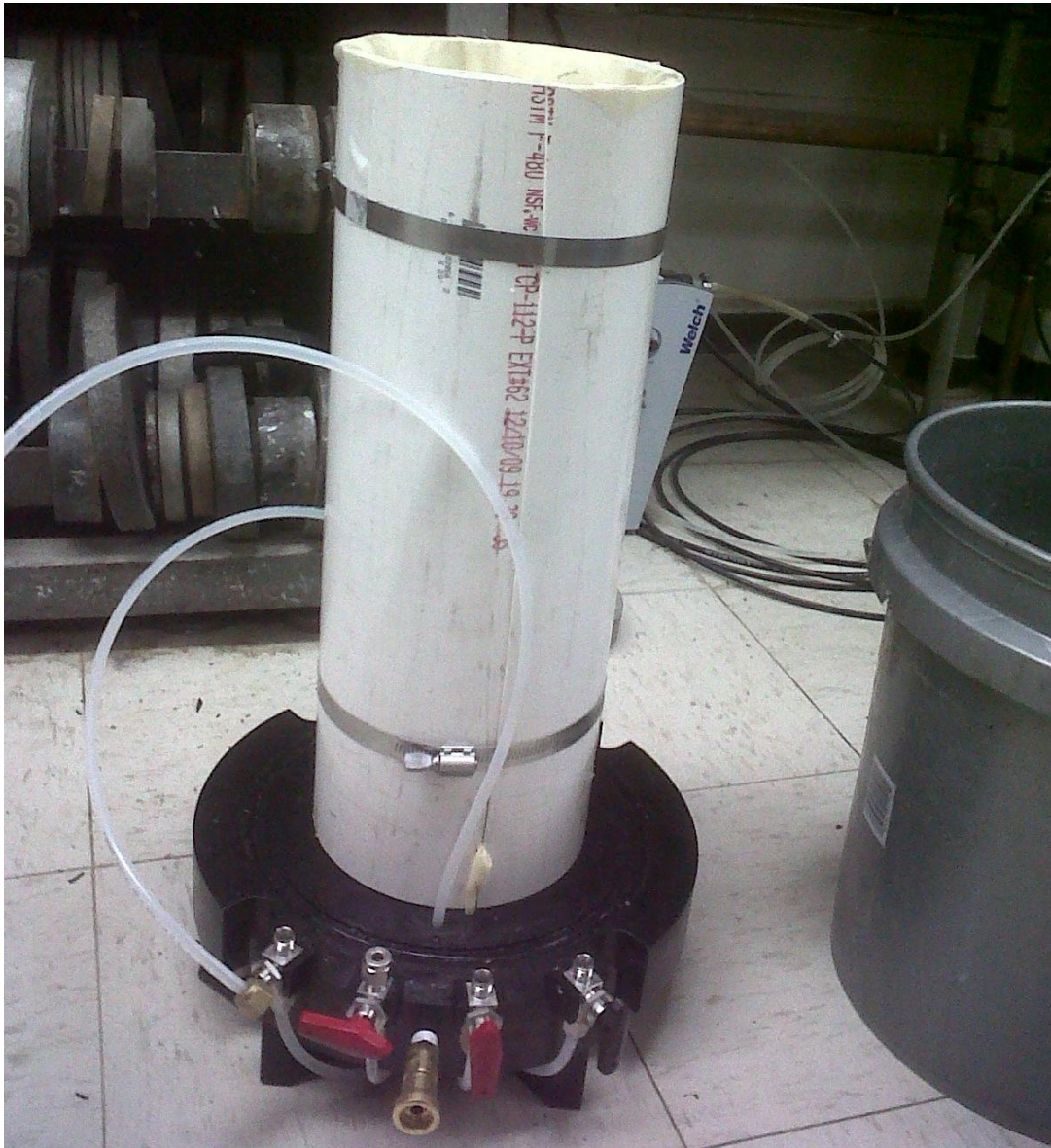
Figure 9.3. PVC forming jacket connected to base.
