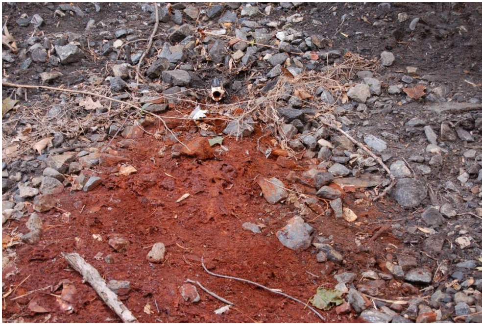
Figure 8.7. Photograph of Port 1 in September 2011. Note the red iron oxide, indicative of excess Fe in the leachate exiting this port.
