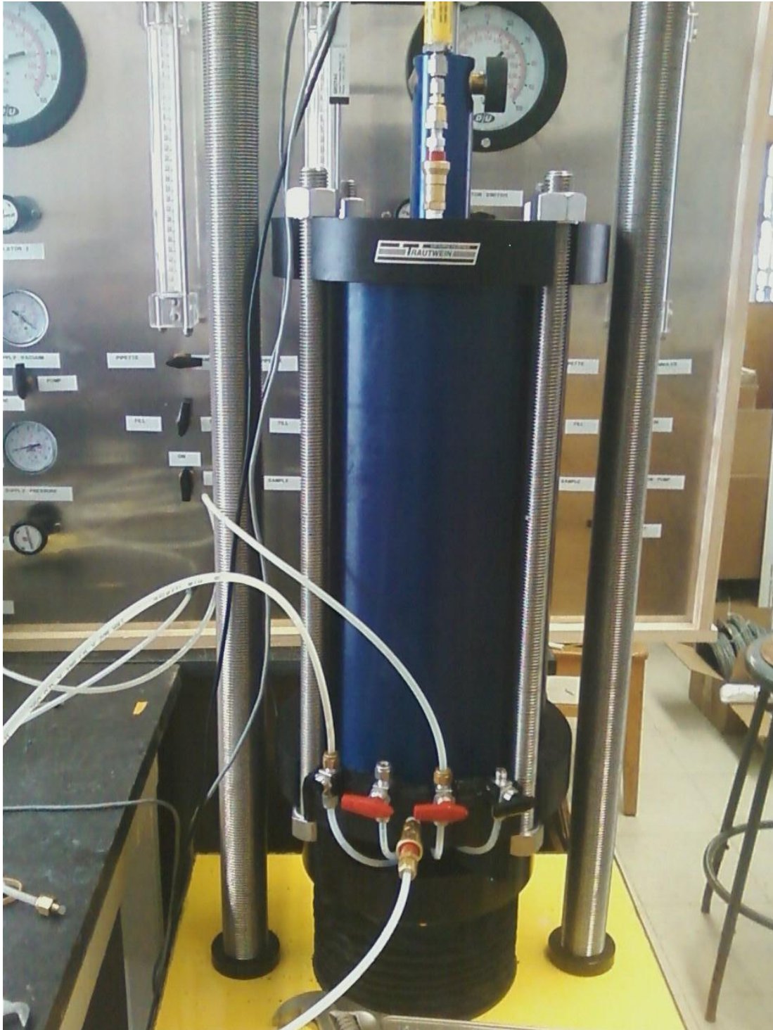
Figure 9.5. Typical sample large capacity triaxial testing device.
