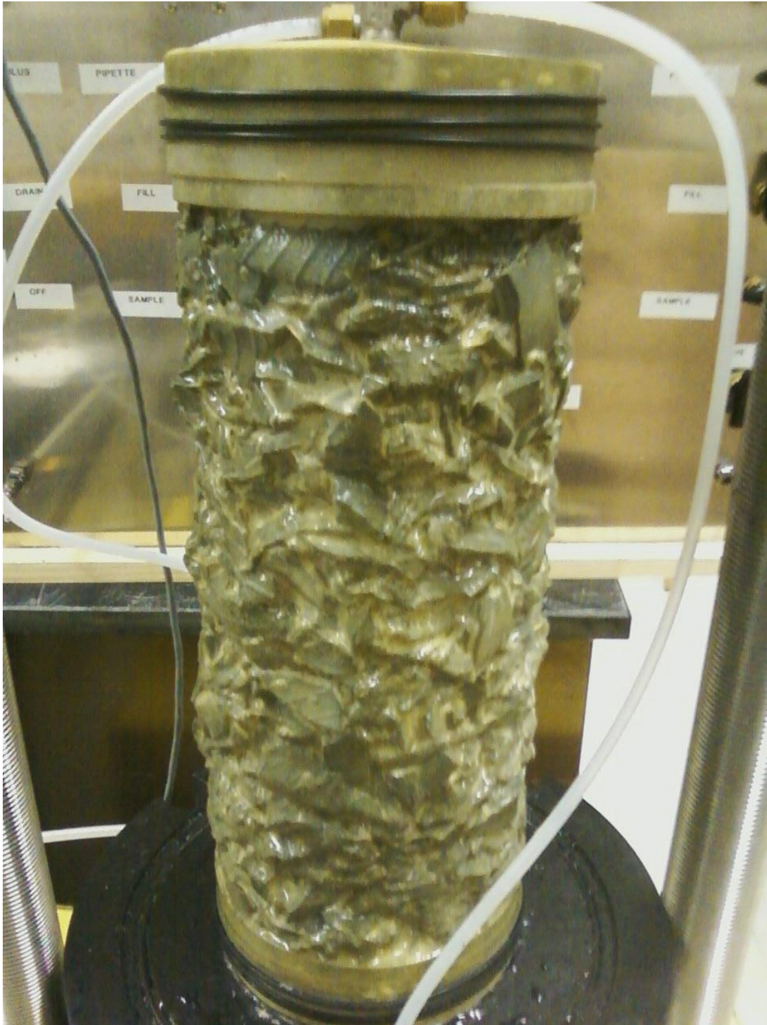
Figure 9.7. Failed sample at 23.0 psi confinement pressure.
