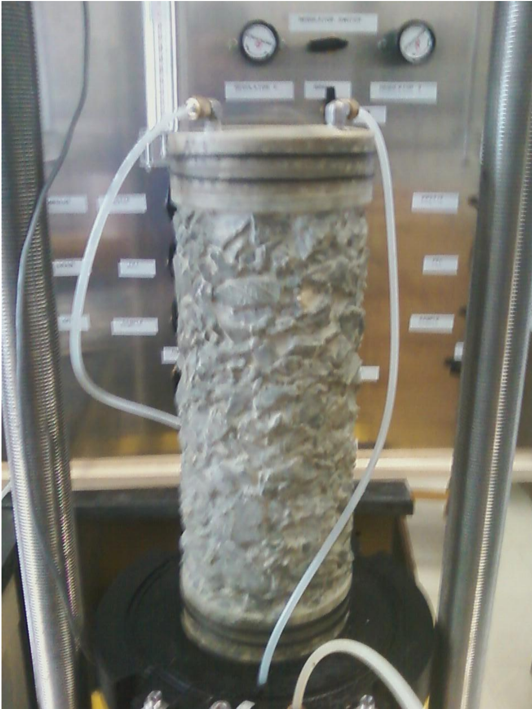
Figure 9.6. Failed sample at 6.5 psi confinement pressure.
