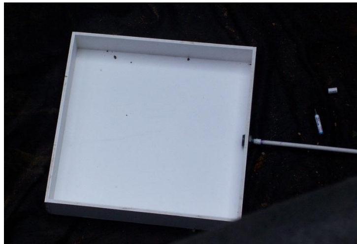
Figure 8.1. Photograph of leachate collection basin and PVC pipe that drained leachate.
