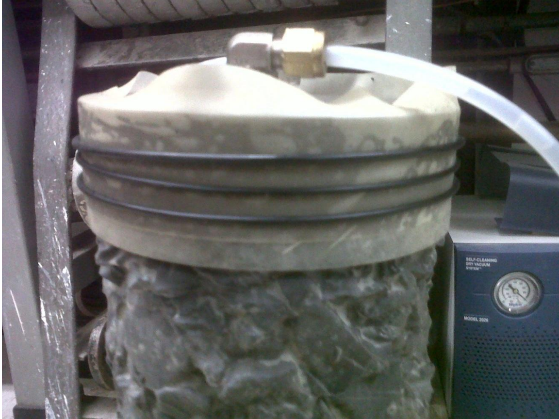
Figure 9.4. Typical sample encased in rubber membrane and sealed with o-rings.
