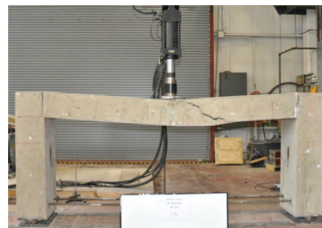
Photo 3 shows the first culvert specimen when it failed. This occurred when the hydraulic actuator reached a force of 58 kips.
