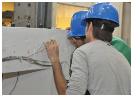
Photo 1 shows Dr. Schumacher and his graduate student Tim Porter looking for cracks in the corner. All cracks are marked to document the progression of cracking with increasing loads.
