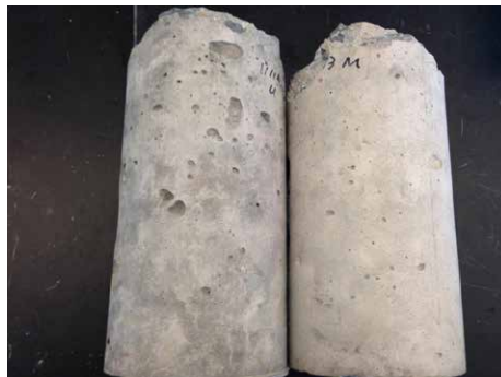
Test cylinders. Left: Cylinder made with ASR-susceptible materials from DelDOT. Right: test cylinders made with the same materials, but with fly ash which makes the concrete more resistant to ASR.
