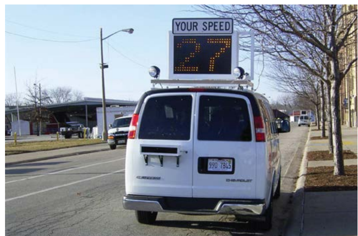
Speed-radar photo enforcement vehicle; enforcement radar unit is mounted on the rear door; down-the-road radar generates the "Your Speed" reading on the rooftop display.
