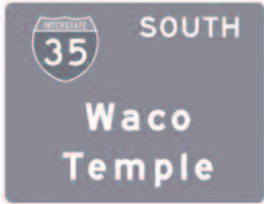
FIGURE 1 Guide sign with Series E Modified lettering, which has served as the standard font.
