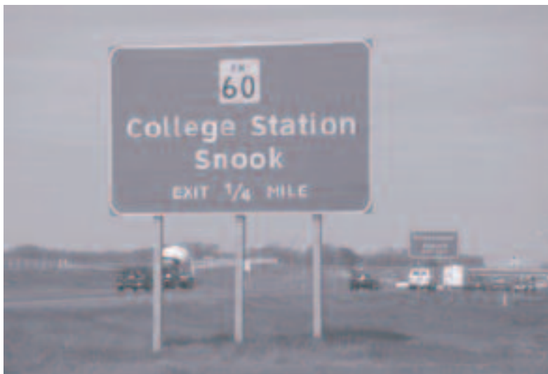
Clearview lettering on highway signs in Texas.
