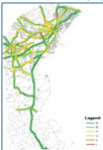
This picture shows one example where GIS can be used for analysis. The roads are color-coded according to their Level of Service (LOS). Images such as above obtained using GIS help in a better understanding of the data.
