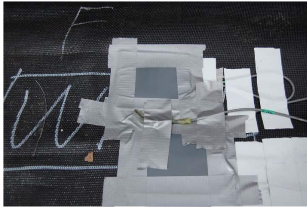
Figure 3.47 Thermistor and its installation
