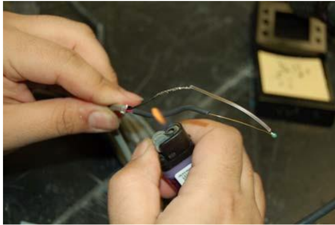
Figure 3.49 Shrinking the heat shrink tubing around the thermistor
