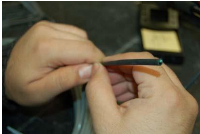
Figure 3.50 Sliding the large diameter heat shrink tubing to cover the thermistor leads
