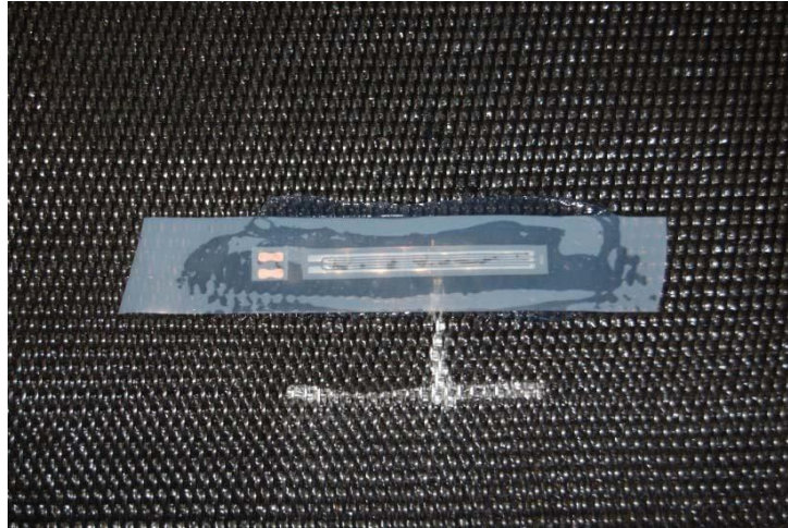
Figure 3.36 Covering the gauge using Teflon tape
