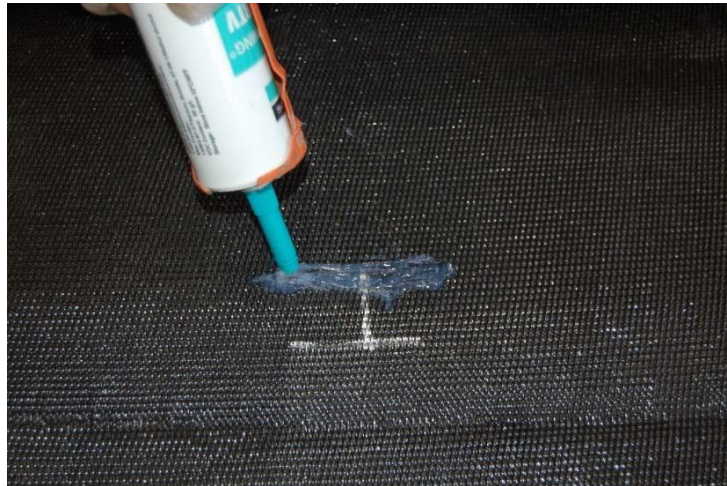
Figure 3.33 RTV application to the geotextile surface
