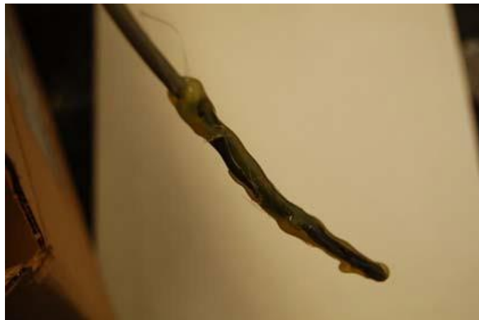
Figure 3.51 Hot glue utilization to waterproof the thermistor
