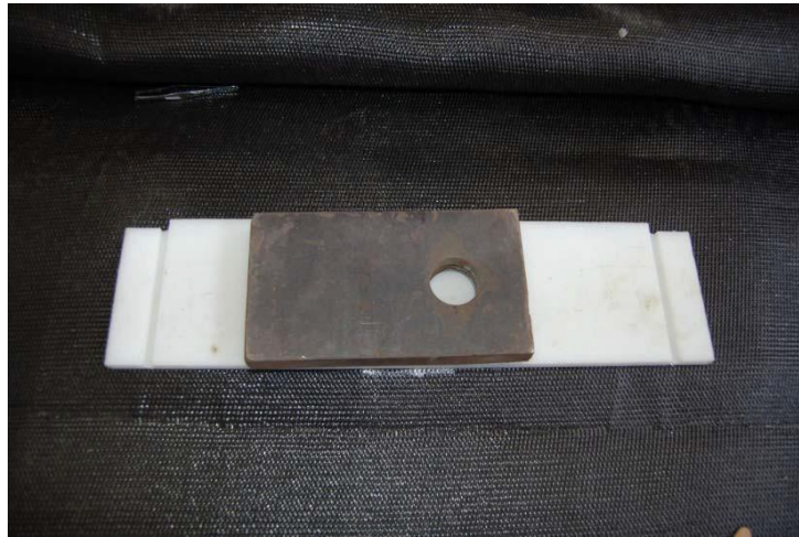
Figure 3.37 Placing a Teflon plate and a weight on the gauge
