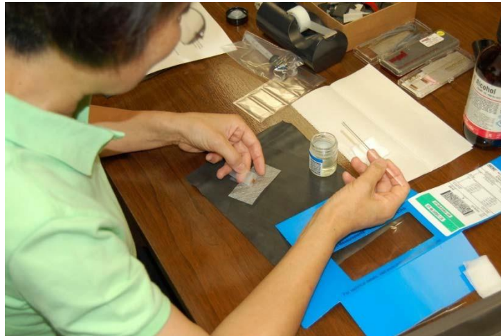
Figure 3.42 Adding epoxy to the ends of the gauge
