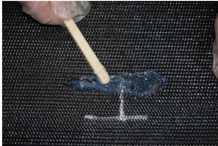
Figure 3.34 RTV smearing out on geotextile
