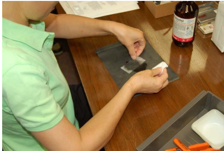
Figure 3.40 Cleaning off the dummy fabric with hydrogen peroxide
