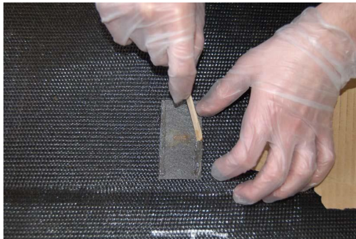
Figure 3.45 Spreading epoxy only on each end of the dummy fabric
