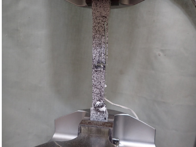
Figure 50. Typical failure mode observed during CFRP tensile testing
