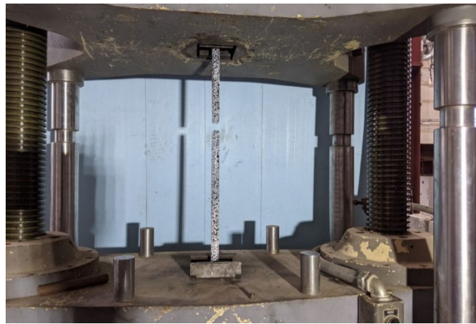
Figure 47. Ruptured rebar tensile test specimen
