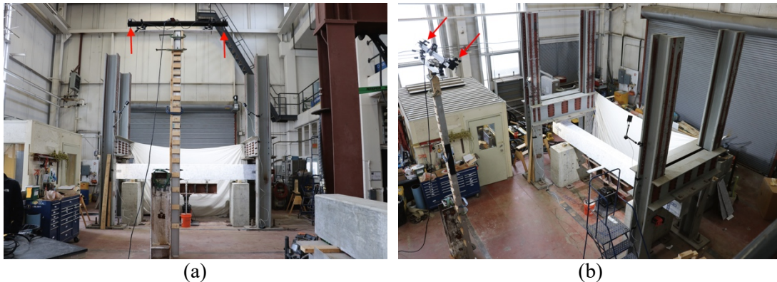
Figure 36. Photographs of the DIC system test (red arrows showing DIC cameras): (a) DIC System placed on top of the aluminum column; (b) Test setup with the DIC system (red arrows showing DIC cameras)
