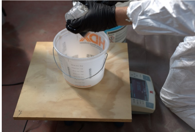
Figure 24. Measuring the weight of the Part A component of the epoxy
