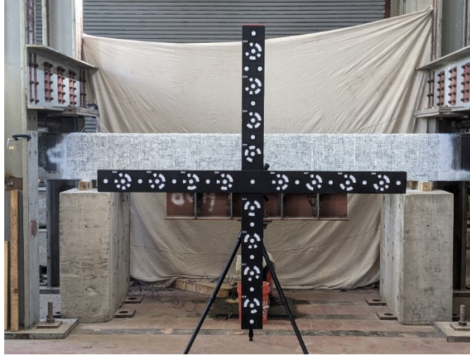
Figure 37. Calibration cross used for the DIC system
