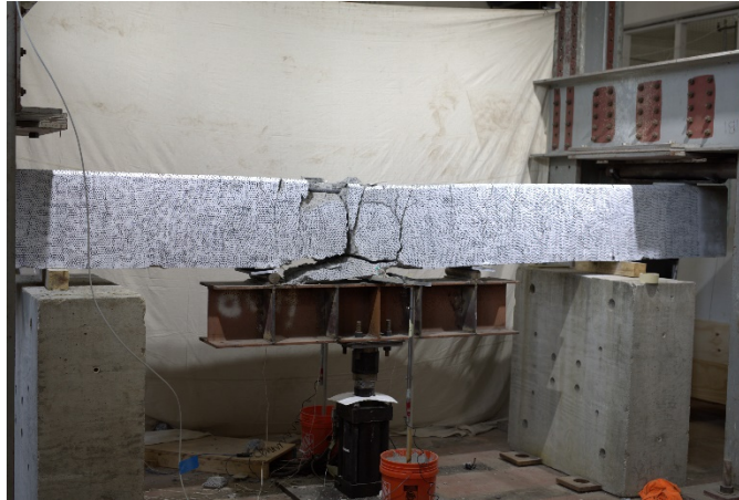
Figure 69. Concrete crushing failure of 0L0U
