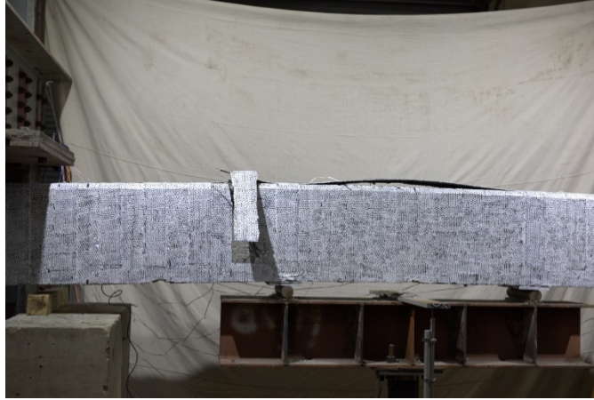
Figure 75. Complete U-Wrap debonding failure of 2L2U-8
