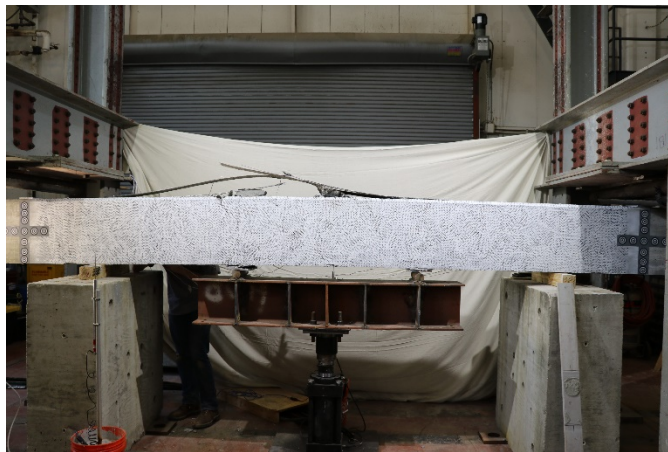
Figure 70. IC debonding failure of 1L0U
