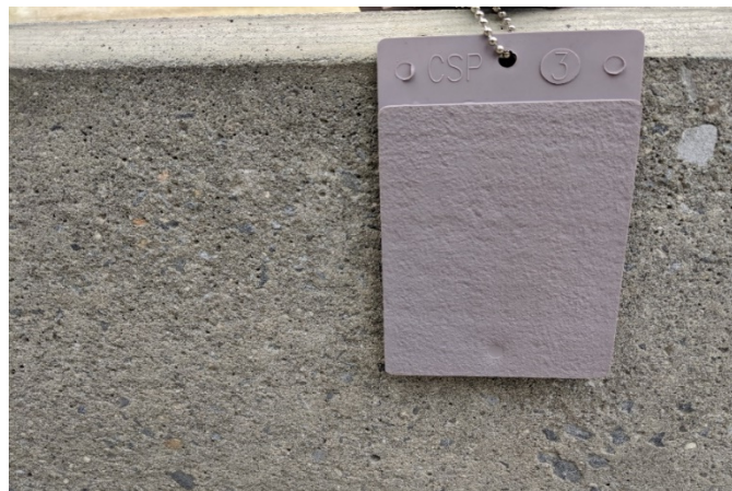
Figure 21. Confirming the CSP of the concrete using an ICRI surface profile coupon
