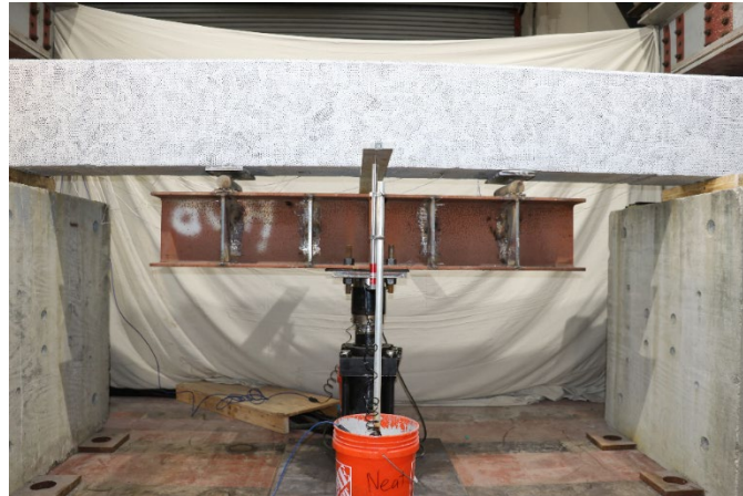
Figure 39. LVDT loaded against the aluminum plate adhered to the girder
