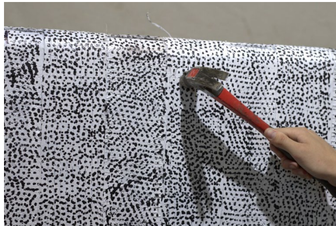
Figure 54. Sounding the U-Wraps to determine whether the U-Wraps are partially debonded
