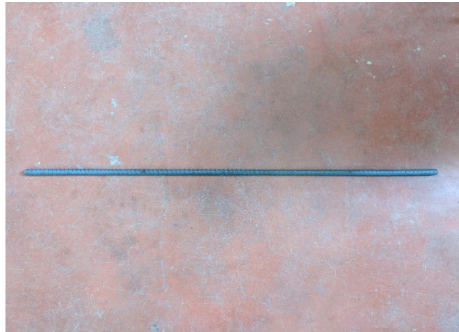
Figure 46. Typical 4-foot section of #6 rebar used for tensile tests
