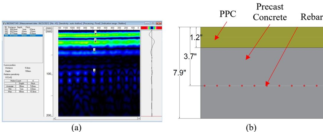
Figure 47. GPR scan in the transverse direction of the bridge deck: (a) GPR scan results; and (b) interpretation of GPR scan results.
