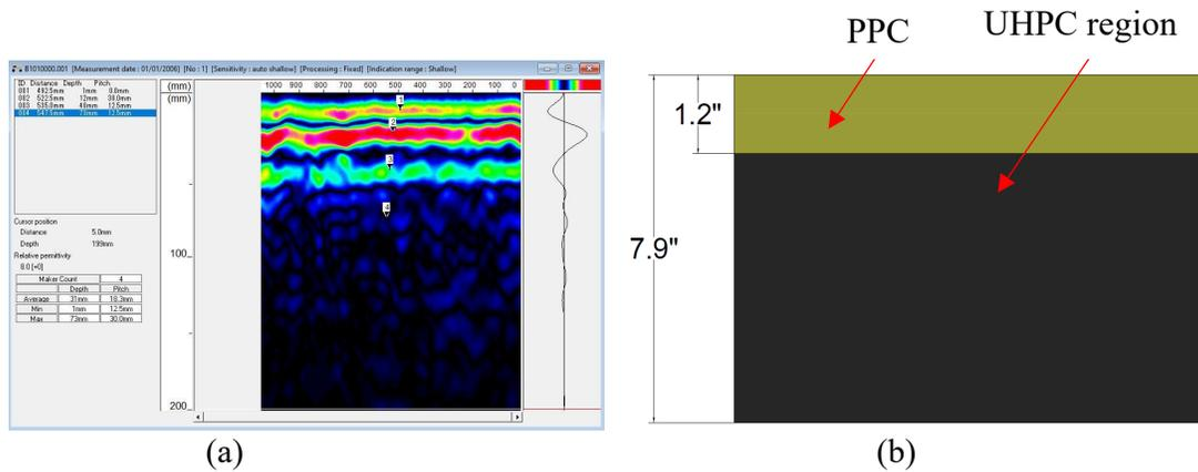
Figure 48. GPR Scan in the transverse direction of the UHPC joint (a) GPR scan results; and (b) interpretation of GPR scan results: no rebar was detected in the UHPC connection.
