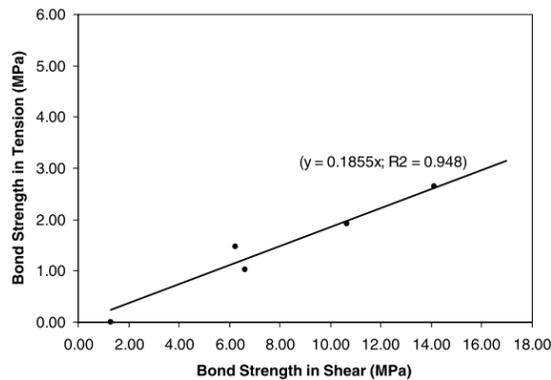
Figure 11. Correlation between bond shear tests and bond pull-off tests concrete (Júlio et al., 2004).
