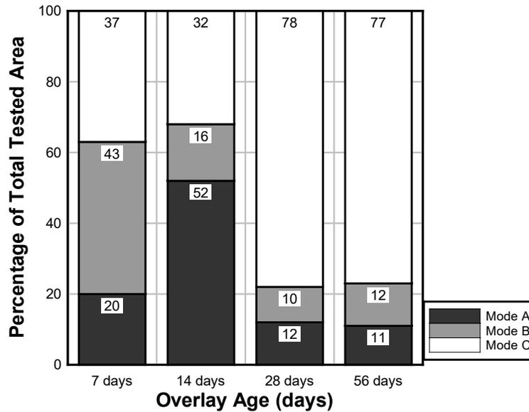
Figure 63. Distribution of PPC overlay failure modes as a function of overlay age.
