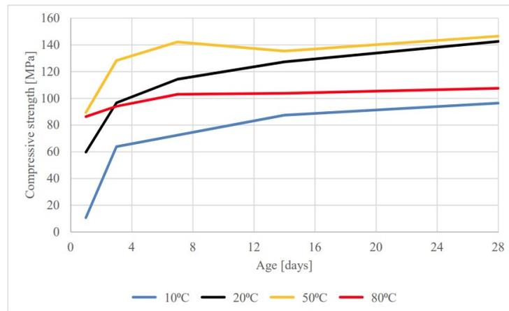
Figure 3. Development of concrete compressive strength at different ambient temperatures (Fladr et al., 2019).
