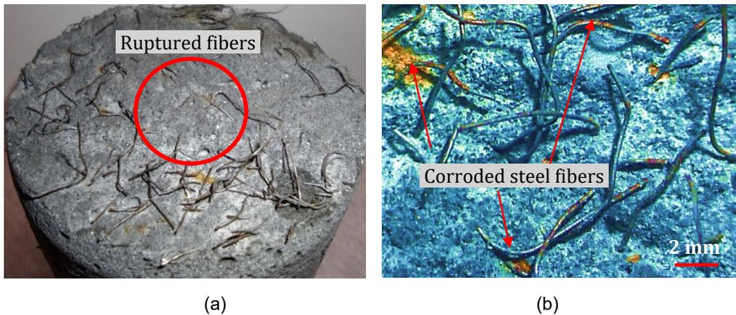
Figure 55. UHPC surface texture following HD: (a) 2-in. core photograph; and (b) stereo microscope photograph. Colors and sharpness were manipulated to highlight corrosion in the microscopic image.
