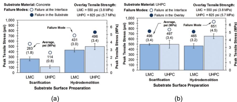
Figure 14. Peak stresses recorded from direct tension bond tests on (a) a concrete substrate, and (b) UHPC substrate (Haber et al., 2017).
