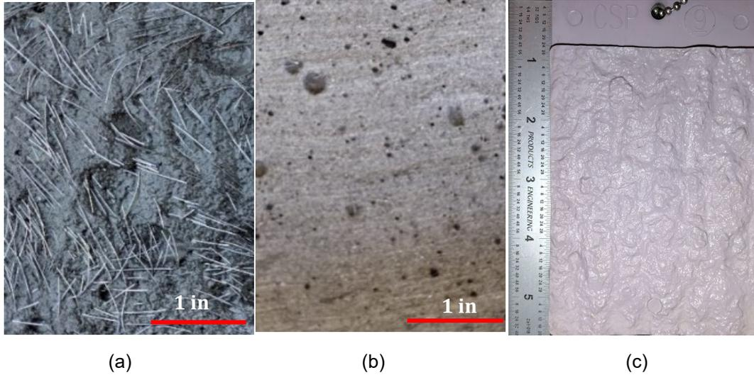
Figure 57. Comparison of UHPC (a) SR and (b) GSB surfaces to (c) an example ICRI CSP chip.
