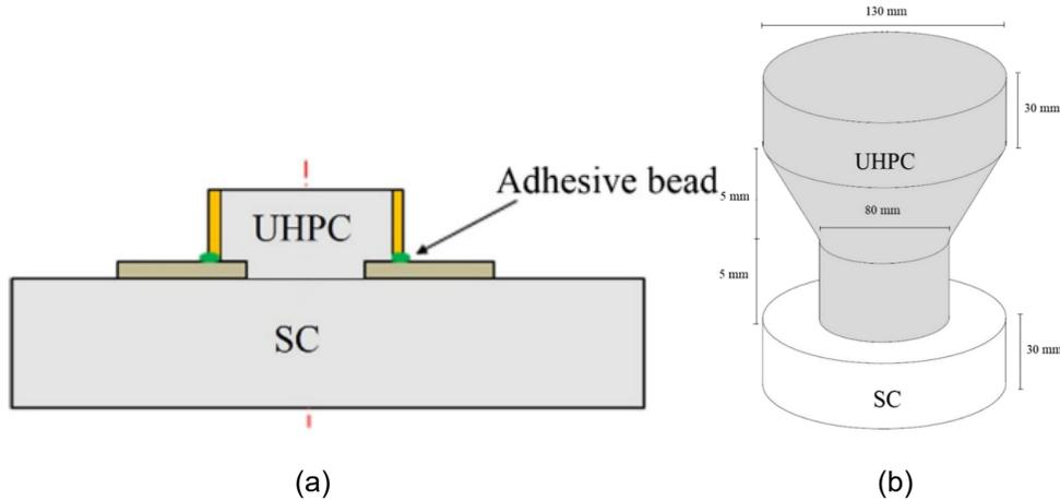
Figure 19. Schematic illustration of (a) the modified bond pull-off test (b) debonding test method (Valipour et al., 2020).
