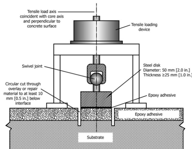
Figure 5. Schematic of the bond pull-off test setup ASTM C1583 (ASTM, 2020).
