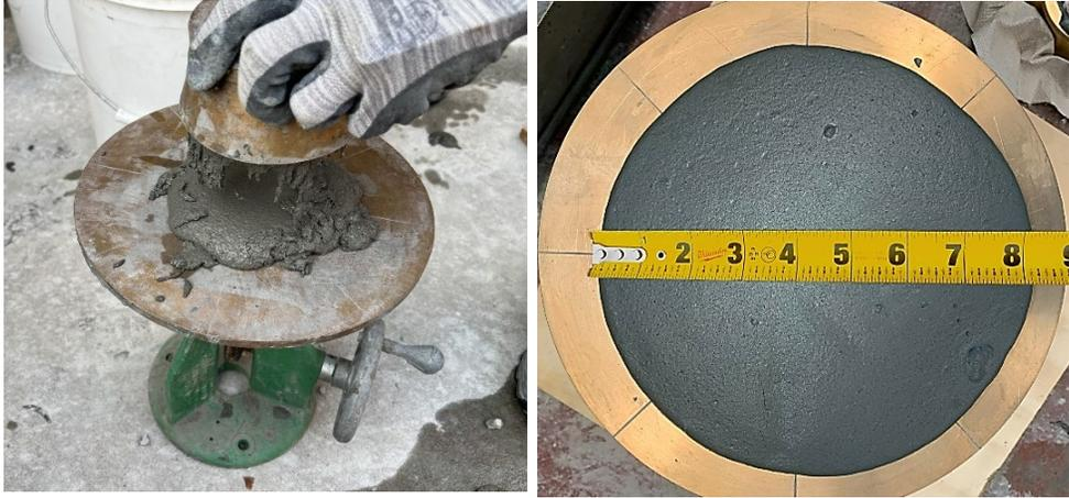
Figure 23. UHPC flow test.
