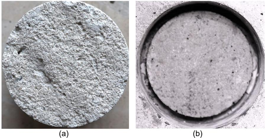
Figure 74. Example of MCD failure Mode B (GSB): (a) core side; and (b) substrate side.
