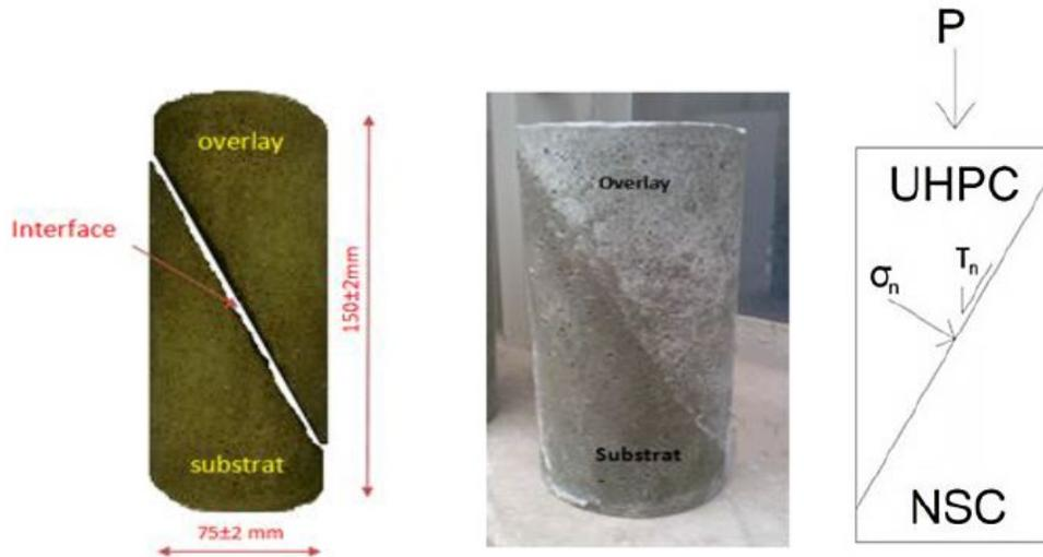
Figure 8. Slant shear bond test specimen (Dawood et al., 2017).
