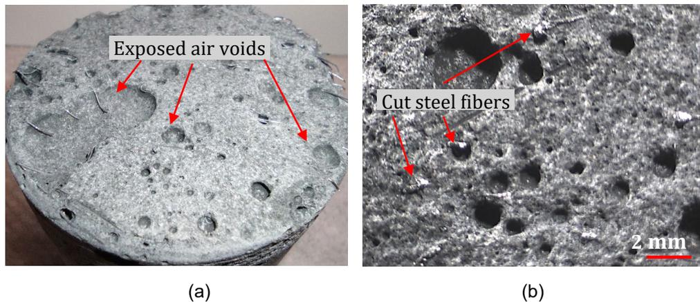
Figure 54. Typical GSB surface: (a) core section photograph; and (b) stereo microscope photograph.
