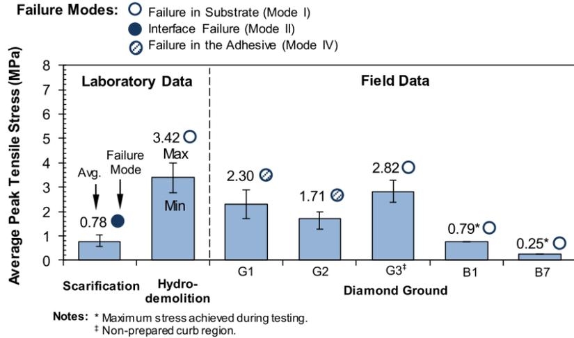
Figure 12. Tensile bond strength of UHPC overlays on concrete (Haber et al., 2018).
