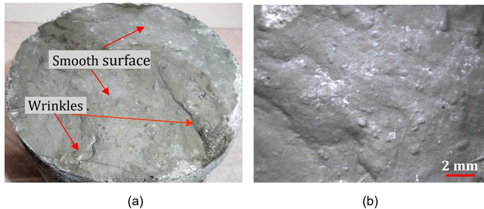
Figure 53. Typical NP surface: (a) core section photograph; and (b) stereo microscope photograph.
