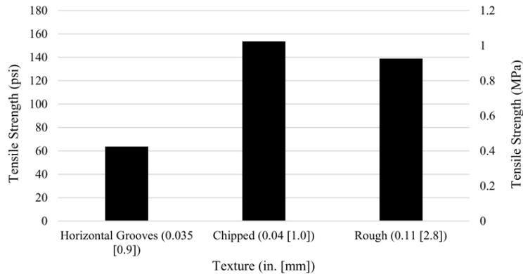
Figure 18. Direct tension bond strength of UHPC overlays on concrete (Newtson et al., 2018).
