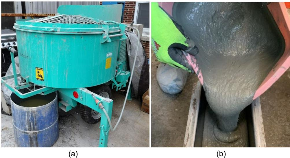
Figure 22. (a) IMER 750 mixer used to mix UHPC; and (b) typical consistency of fresh UHPC.
