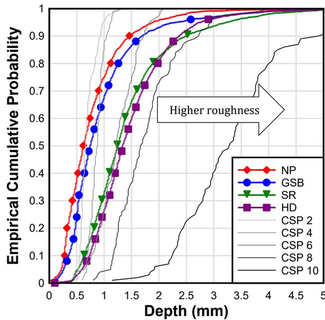
Figure 59. Surface profile gauge empirical cumulative probability functions for the different surface preparation methods.
