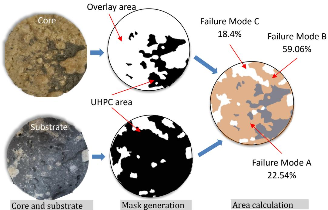
Figure 38. The process of calculating areas of each failure mode. This example is for a PPC overlay with a coring depth of 0.5 in.
