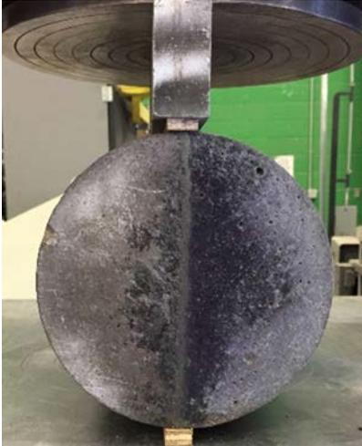
Figure 7. Splitting tensile bond test setup (Newtson et al., 2018).
