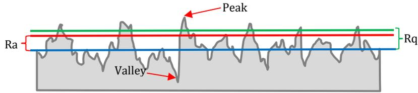
Figure 35. Illustration of Ra, Rq, Peaks, and valleys of a surface.
