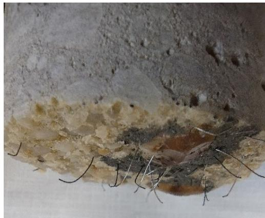
Figure 72. Example failure mode showing steel fibers from UHPC embedded in PPC.
