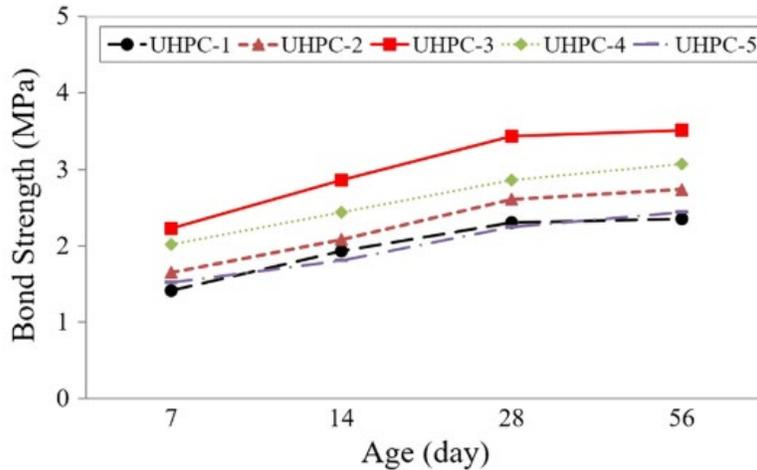
Figure 20. Effect of curing of UHPC overlay on bond strength (UHPC 1,2,3,4, and 5 represent different mix ratios) (Valipour et al., 2020).
