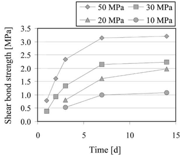
Figure 4. Interface shear bond strength development for overlays of different compressive strengths (Bissonnette et al., 2011).
