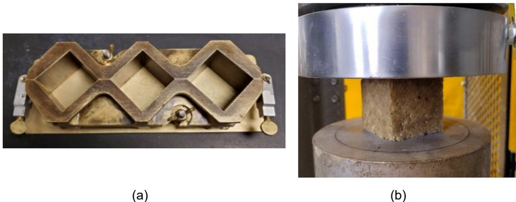
Figure 25. (a) 2-in. brass cube mold; and (b) compressive test on a 2-in. PPC cube.
