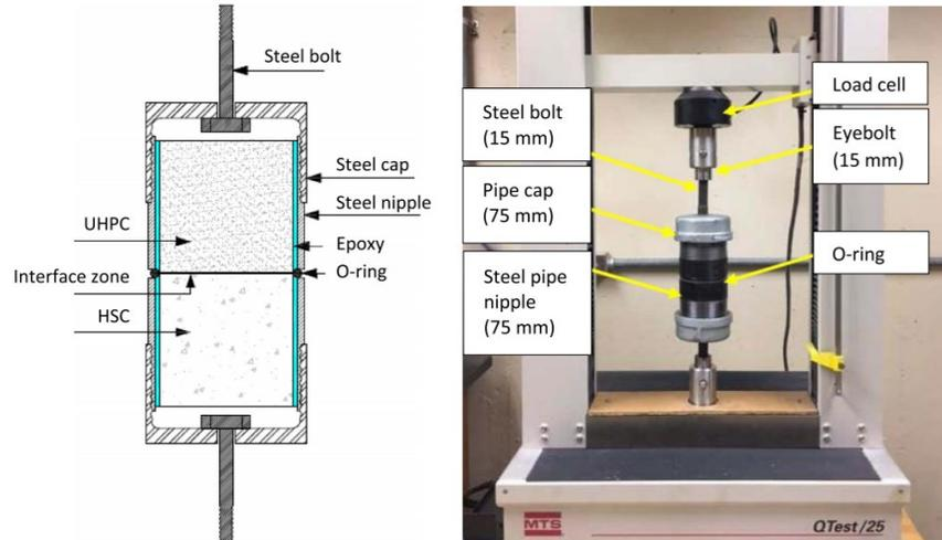
Figure 6. Example specimen for direct tension bond tests (Semendary et al., 2019).
