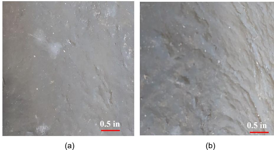
Figure 30. Elephant skin on NP UHPC surface: (a) smooth surface, (b) wrinkles near the formwork edges/corners.
