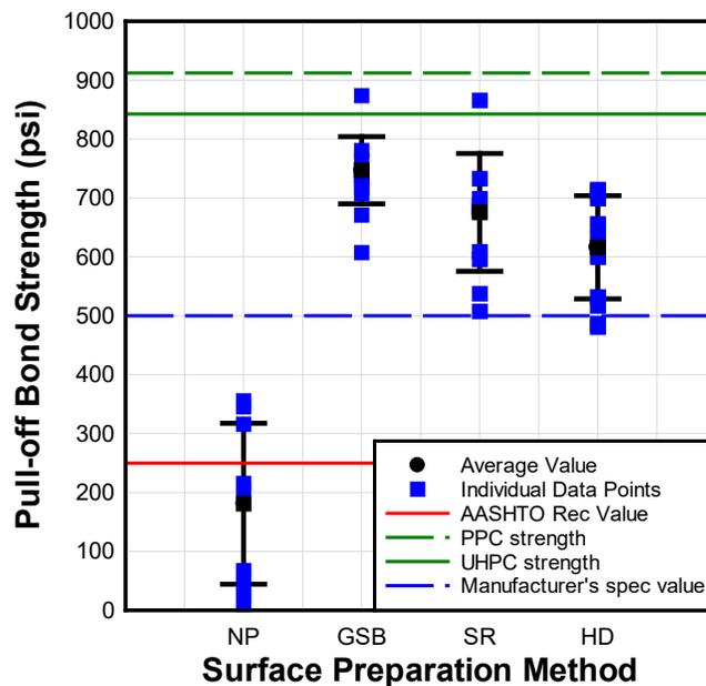
Figure 69. PPC bond pull-off strength as a function of surface preparation method. Error bars indicate one standard deviation.
