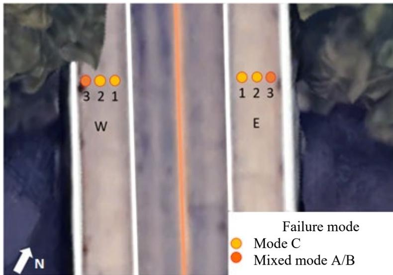
Figure 77. Specimen locations and failure modes. 'W' indicates west shoulder and 'E' indicates east shoulder.
