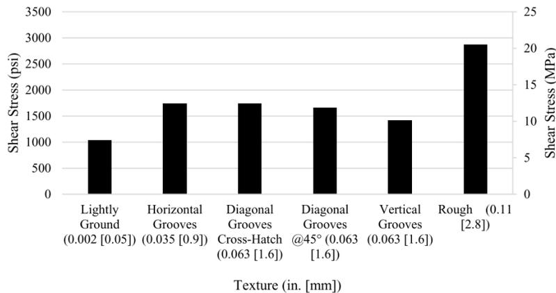
Figure 16. Slant-shear bond strengths (Newtonson et al., 2018).
