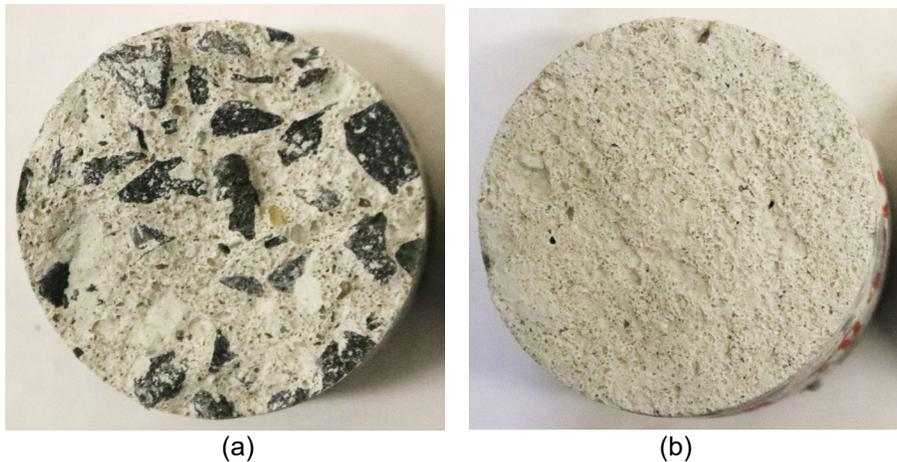
Figure 66. Typical MCD failure modes: (a) Mode C (core from cohesive tensile strength test, i.e., no UHPC substrate); and (b) Mode B observed for all tests on MCD-UHPC bonded specimens indicating lack of coarse aggregates within the weak interphase.
