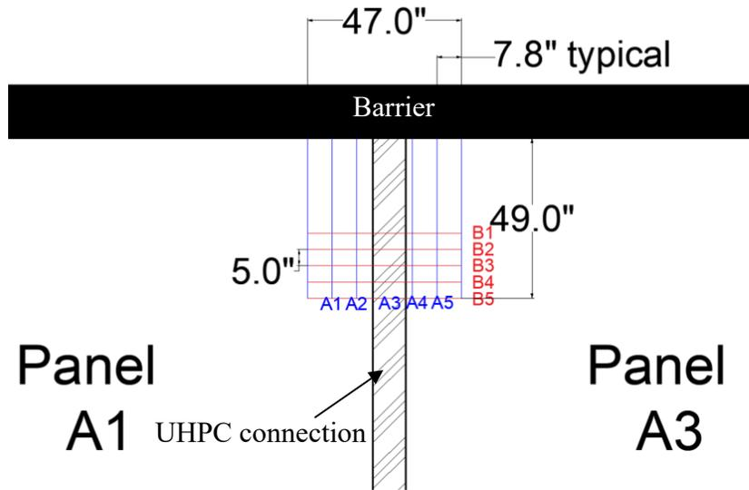
Figure 46. Plan view of the bridge showing GPR scanning location. Scan direction is from A1 to A5 and from B5 to B1.
