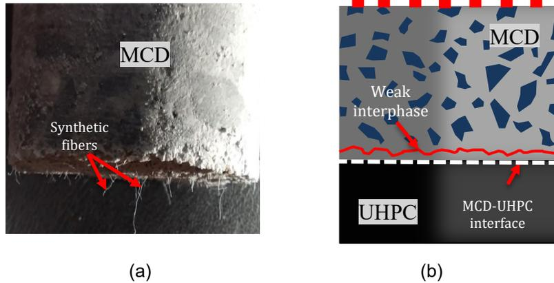
Figure 65. (a) Failed MCD specimen, (b) illustration of the weak interphase at the MCD-UHPC interface.
