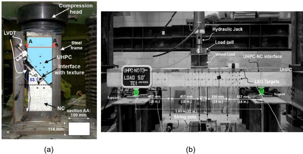
Figure 9. Test specimens: (a) slant shear bond test; and (b) flexural test on a precast concrete deck with UHPC overlay (Aaleti et al., 2019).
