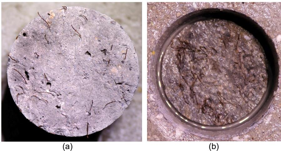
Figure 76. Example of LMC failure Mode B (HD), (a) core side; and (b) substrate side.
