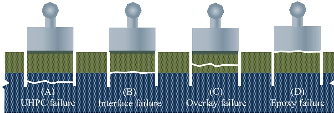
Figure 37. Schematic of possible failure modes.
