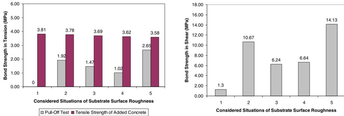
Figure 10. Tensile bond strength of concrete-to-concrete bonds (Júlio et al., 2004).
