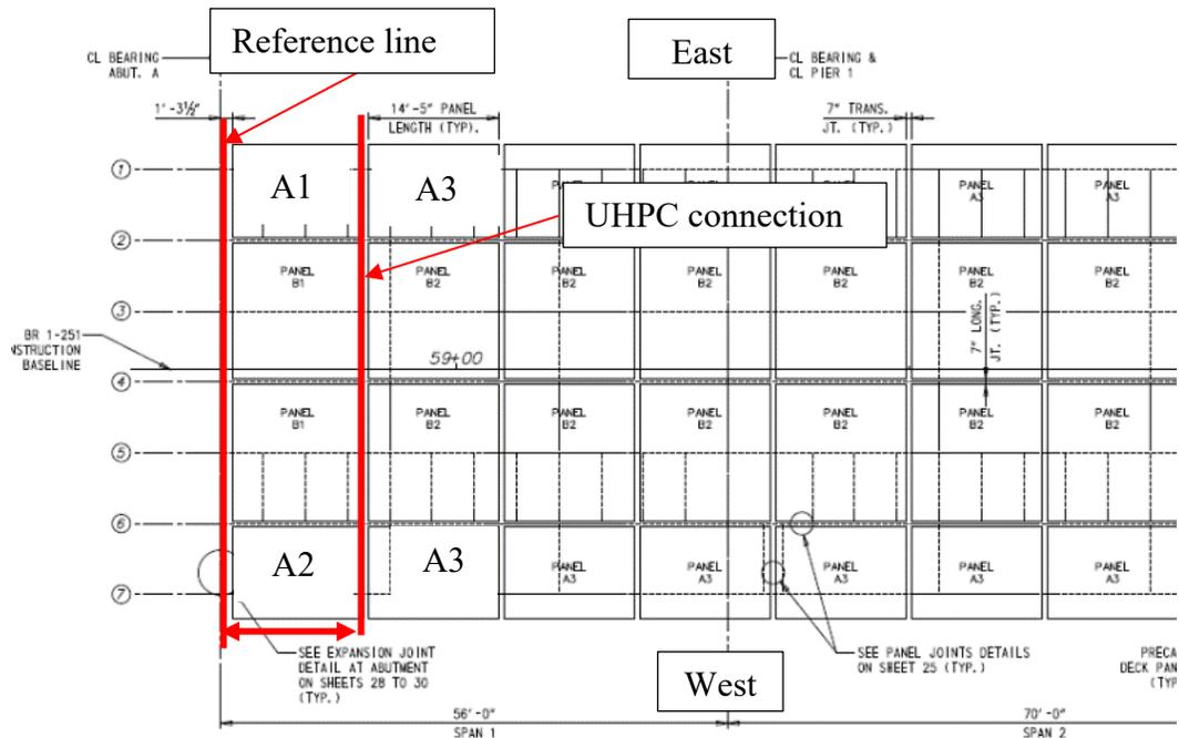
Figure 44. Plan view of the deck panel layout with the expansion joint as reference line.
