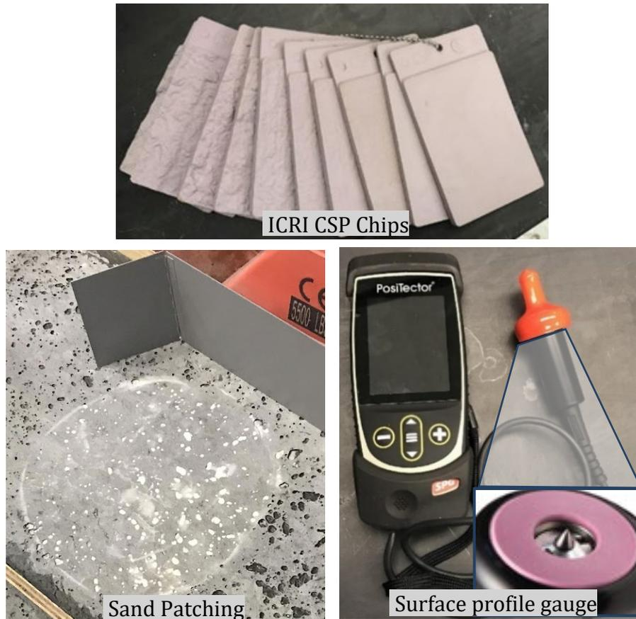
Figure 34. Roughness measurement methods.
