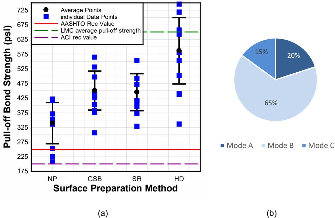
Figure 75. (a) LMC bond pull-off strengths as a function of surface preparation method; and (b) failure mode distribution of LMC for the HD method. Error bars indicate one standard deviation.
