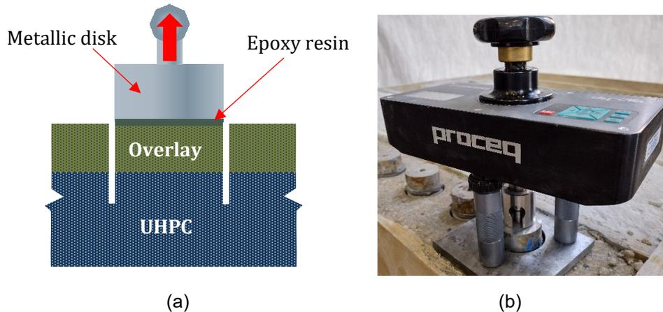
Figure 36. (a) Bond pull-off test schematic; and (b) Proceq DY-216 bond pull-off tester.
