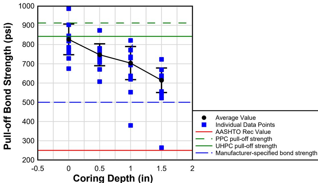
Figure 60. Bond pull-off strength data for PPC as a function of coring depth. Error bars indicate one standard deviation.
