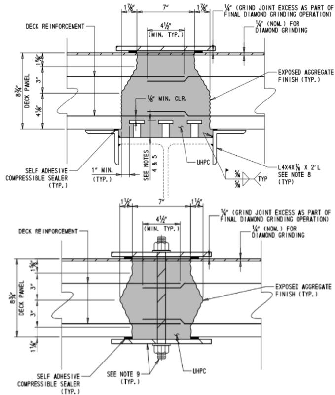
Figure 41. Longitudinal and transverse joint details as presented in BR 1-251 plans.
