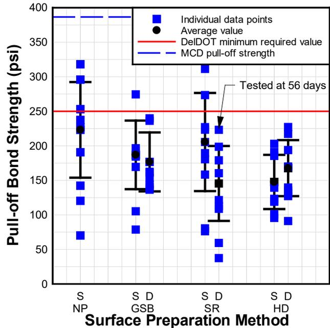
Figure 73. MCD bond pull-off strengths as a function of surface preparation method. ‘S’ and ‘D’ respectively indicate SSD and Dry substrates. Error bars indicate one standard deviation.
