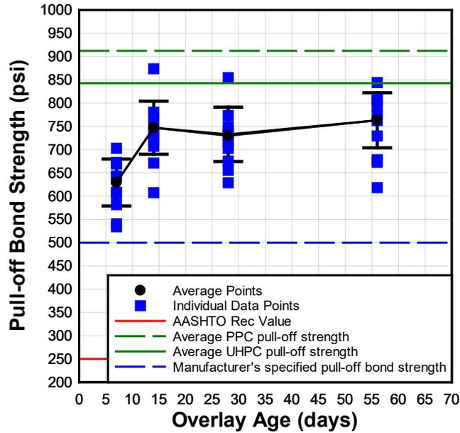
Figure 62. PPC bond pull-off strength as a function of overlay age. Error bars indicate one standard deviation.
