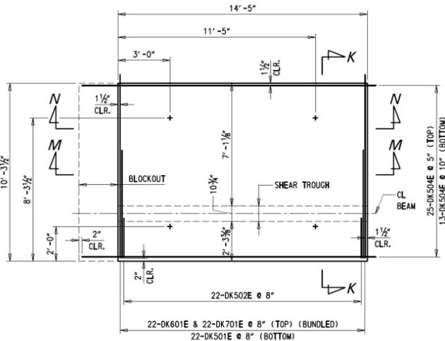
Figure 50. Joint details of deck panel.
