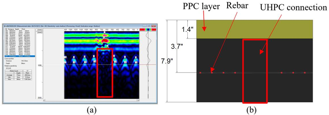
Figure 49. GPR scan in the longitudinal direction in UHPC joint: (a) GPR scan results; and (b) interpretation of GPR scan results: no rebar was detected within the UHPC joint.
