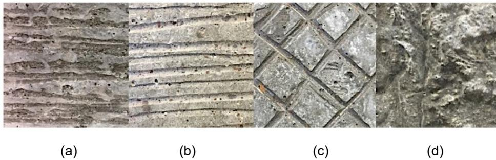
Figure 15. Surface texture of the substrate: (a) lightly ground with a depth of 0.002 in. (0.05 mm); (b) horizontal grooves with a depth of 0.035 in. (0.9 mm); (c) cross-hatched with a depth of 0.063 in. (1.6 mm); and (d) rough with a depth of 0.11 in. (2.8 mm) (Newtonson et al., 2018).
