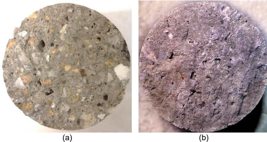
Figure 68. Typical LMC failure modes: (a) Mode C (core from cohesive tensile strength test, i.e., no UHPC substrate); and (b) Mode B observed for all tests on LMC-UHPC bonded specimens.
