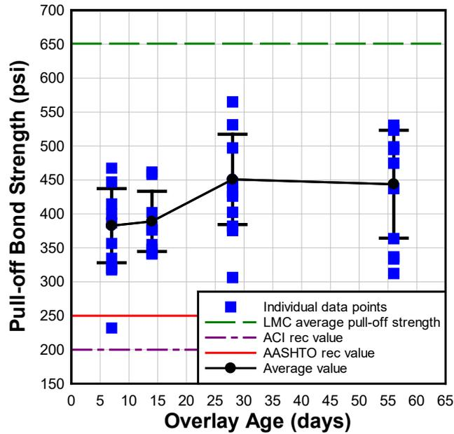
Figure 67. LMC bond pull-off strength as a function of overlay age. Error bars indicate one standard deviation.
