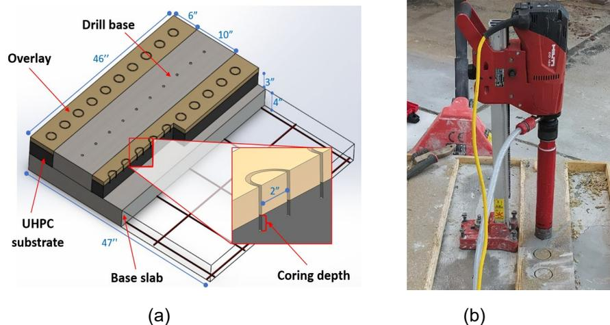
Figure 21. (a) Illustration of the slab components and substrate details; and (b) drill anchored to the drill base.
