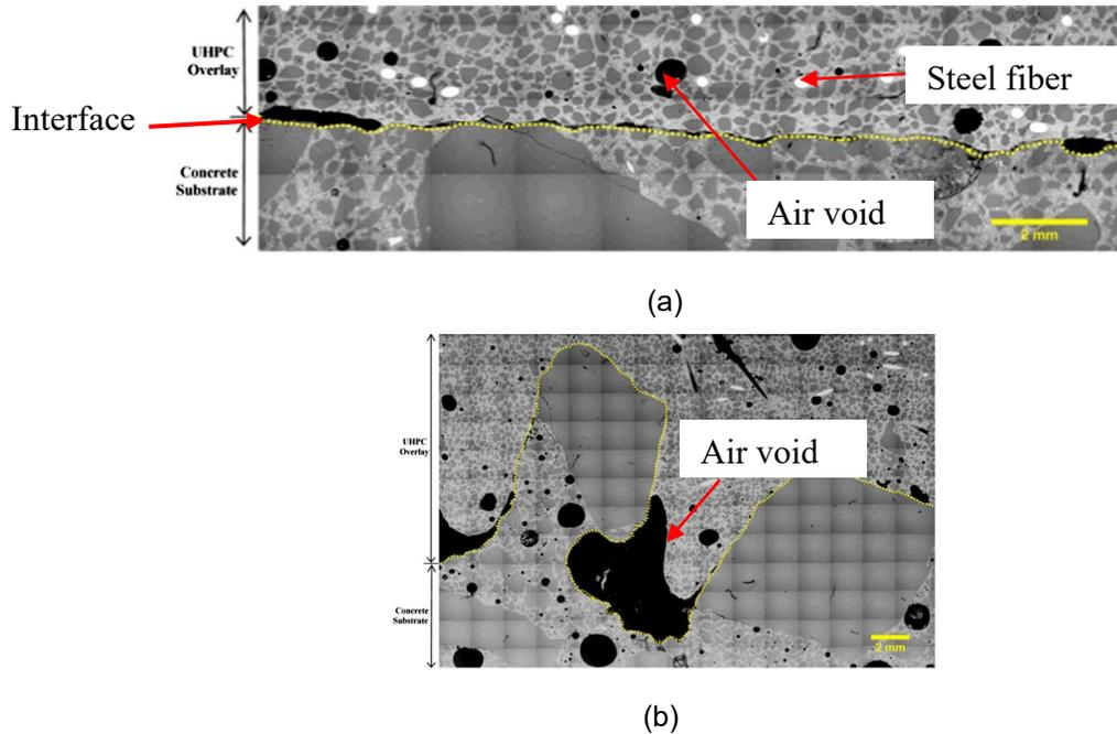
Figure 13. Microstructure of the interface region for specimens prepared via (a) scarification and (b) hydrodemolition (Haber et al., 2018).
