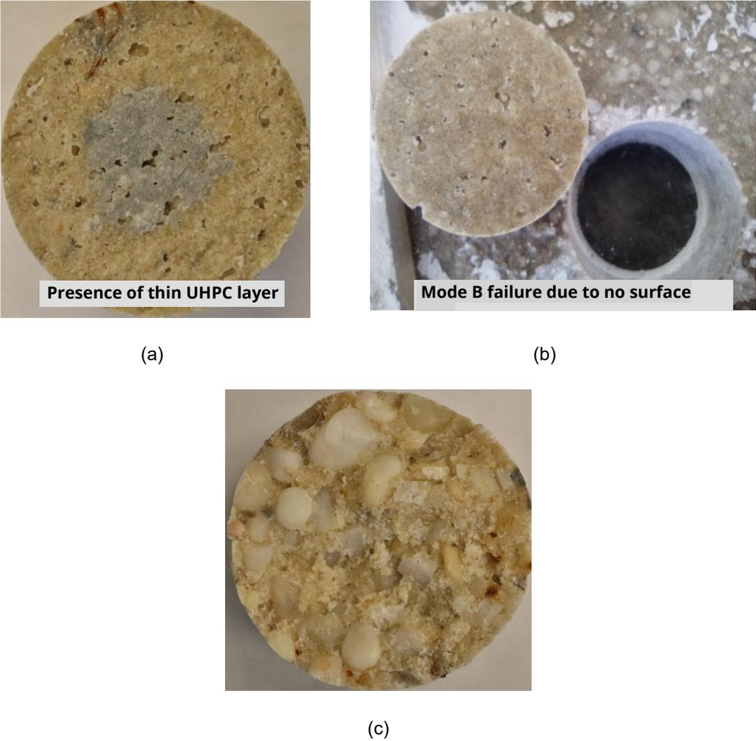
Figure 70. Typical failure modes observed for PPC overlay: (a) mixed failure Mode A and B (core side); (b) failure mode B (core and substrate side); and (c) failure Mode C (core side).
