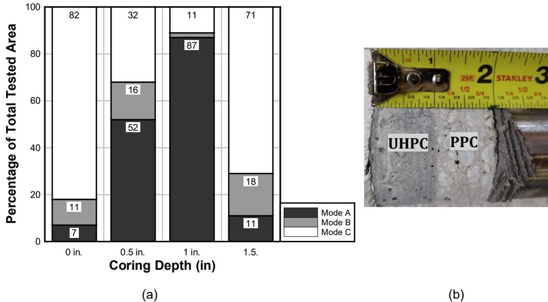
Figure 61. Failure mode of PPC overlay: (a) distribution of failure modes at different coring depths; and (b) example of Mode A failure from a 1-in. core depth sample.
