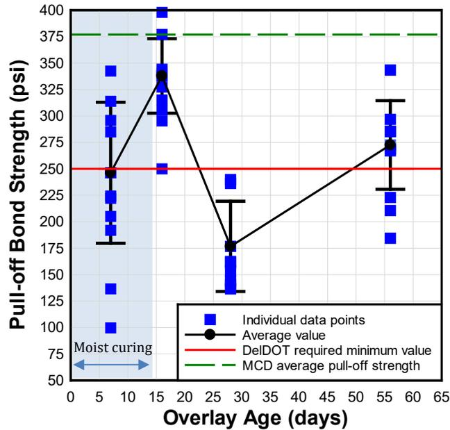
Figure 64. MCD overlay bond pull-off strength as a function of overlay age. Error bars indicate one standard deviation.
