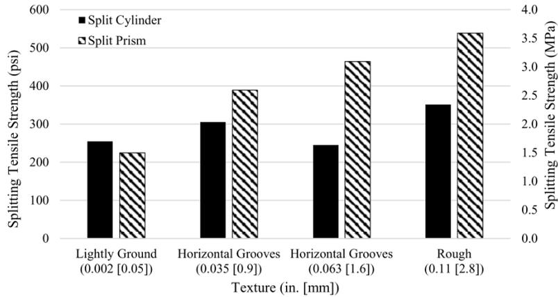
Figure 17. Split cylinder and split prism bond test results (Newtson et al., 2018).
