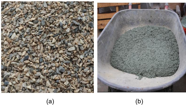
Figure 28. (a) Delaware #8 aggregate used for LMC; and (b) freshly mixed LMC.
