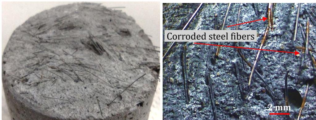
Figure 56. UHPC surface texture following SR: (a) 2-in. core photograph; and (b) stereo microscope photograph. Colors and sharpness were manipulated to highlight corrosion in the microscopic image.
