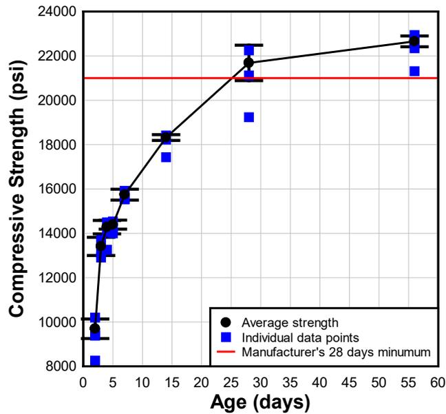
Figure 24. UHPC strength gain over time. Error bars indicate one standard deviation.
