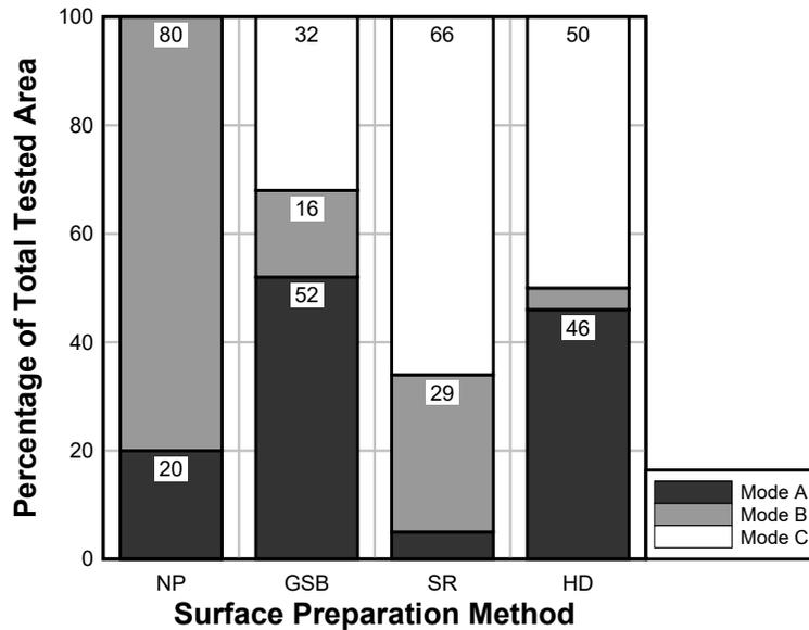
Figure 71. Distribution of PPC failure modes as a function of surface preparation method.
