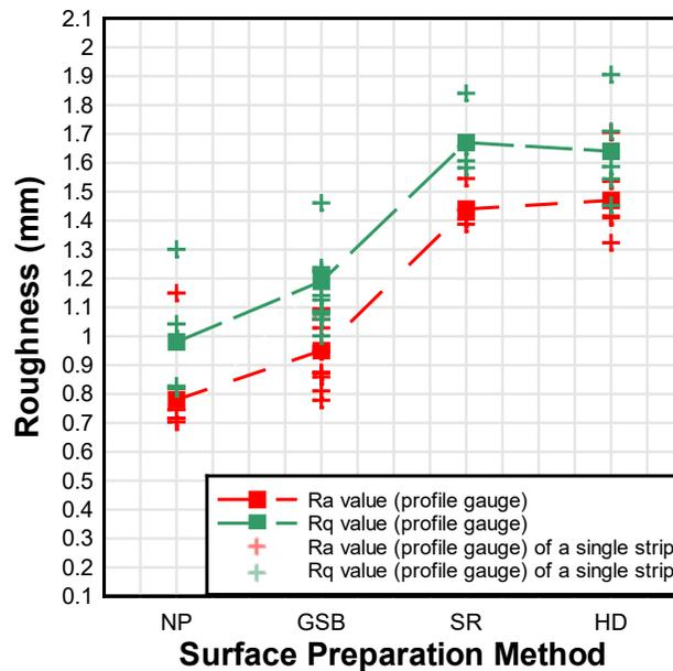
Figure 58. Surface profile gauge roughness measurement results for the different surface preparation methods.
