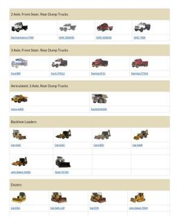
types, including 2-axle, 3-axle, and articulated, off road trucks. Six backhoes and six dozers are illustrated. Then there are four motor graders, three hydraulic excavators, and seven loader configurations. A cold planer (milling machine), a recycler/reclaimer (think full-depth reclamation), a vibratory roller, three scrapers (aka, "pans"), and a transfer/shuttle buggy (sometimes used to support asphalt paving operations) are also featured.
