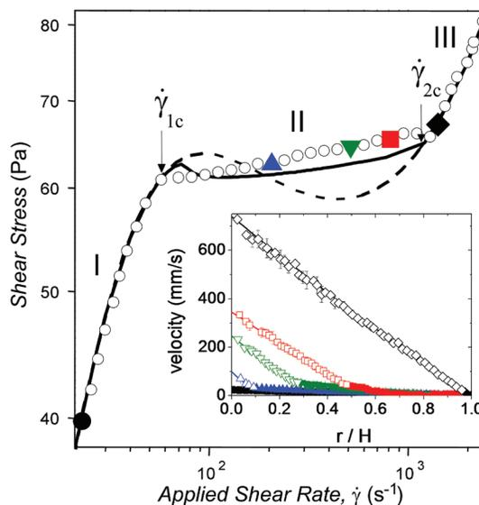
FIGURE 1: Steady state rheology of shear banding CTAB wormlike micelles [3, 5]. Open circles: data, curves: model. Inset: velocity profiles vs. relative position ( $r/H$ ) for region (II),  $\dot{\gamma}_{1c} < \dot{\gamma}_0 < \dot{\gamma}_{2c}$  are characteristic of shear banding. The data point colors and shapes correspond to points in the outer graph. Closed and open symbols represent points in the low-shear band (I) and high-shear band (III), respectively.
