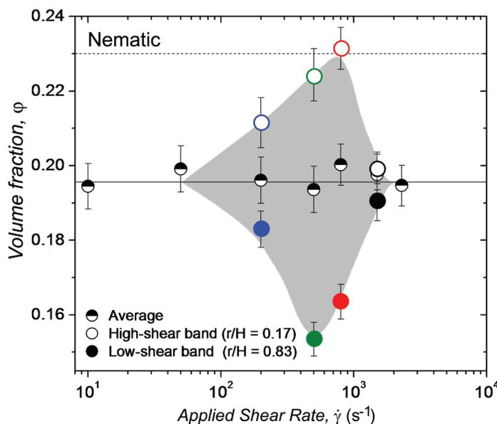
FIGURE 3: Measured CTAB volume fractions for the gap positions,  $r/H$ , indicated, indicating flow-concentration coupling during shear banding (shaded region). Solid and dashed lines give the concentration of the fluid at rest and that of an equilibrium nematic phase, respectively. Symbol colors correspond to the applied shear rates in previous figures.
