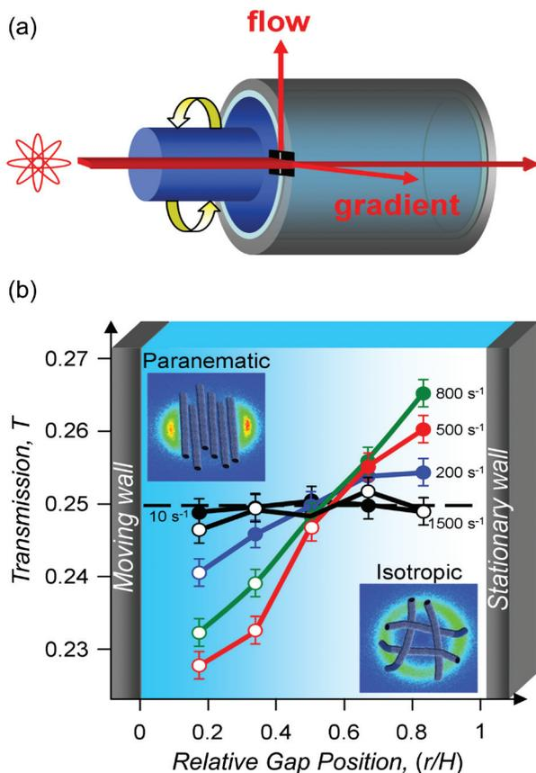
FIGURE 2: (a) Schematic of the SNAFUSANS shear cell, indicating the incident beam direction relative to the beam slit (black). (b) Absolute neutron transmission ( $T$ ) profiles for shear banding CTAB wormlike micelles confirm the existence of flow-concentration coupling. Insets show 2D SANS profiles for positions in the high-shear (paranematic) and low-shear (isotropic) bands.
