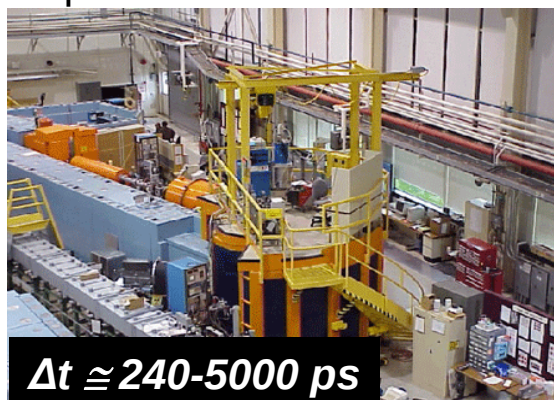
NG2 Backscattering spectrometer
