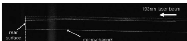
Fig. 2. Formation of microchannels at the exit face [1].
