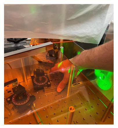
a. To mode lock the oscillator, *carefully* remove the rectangular piece orange acrylic covering the cavity on the far right (closest to the laser). *Carefully*, insert your hand to reach the translation stage holding a prism closest to the laser. DO NOT TOUCH THE BEAM! Grip the stage and pull backward so the stage is shifted. The oscillator is mode locked when the oscilloscope shows a stable pattern of pulsed waves (see below).
