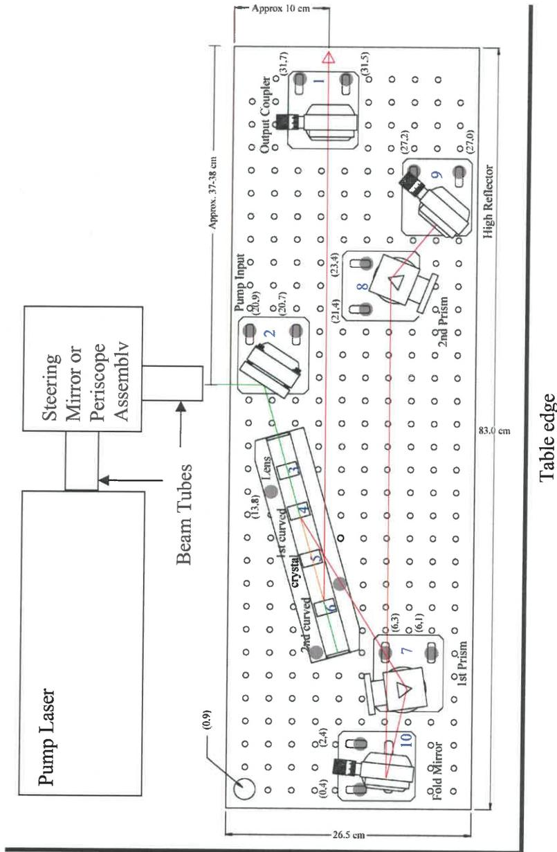
**Figure 5.2:** Basic layout of the laser, including number designations for the optics, and screw coordinate positions for the mounts. Alternate pump laser configurations are shown in Figure 5.3.
