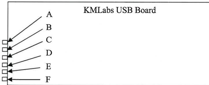
Figure 9.1: Location of the SMA connectors on the KMLabs USB board.
