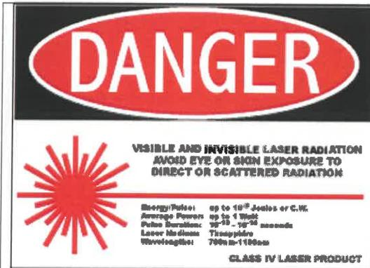
**Figure 3.1:** Danger label, with specifications located near the exit aperture.
