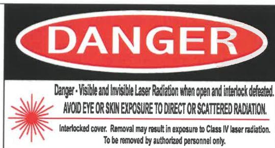
**Figure 3.4:** Interlocked cover label affixed on the side panel, just below the lid-handle.
