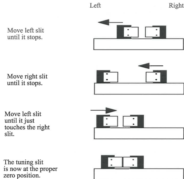
**Figure 8.1: Tuning slit setup procedure.**
