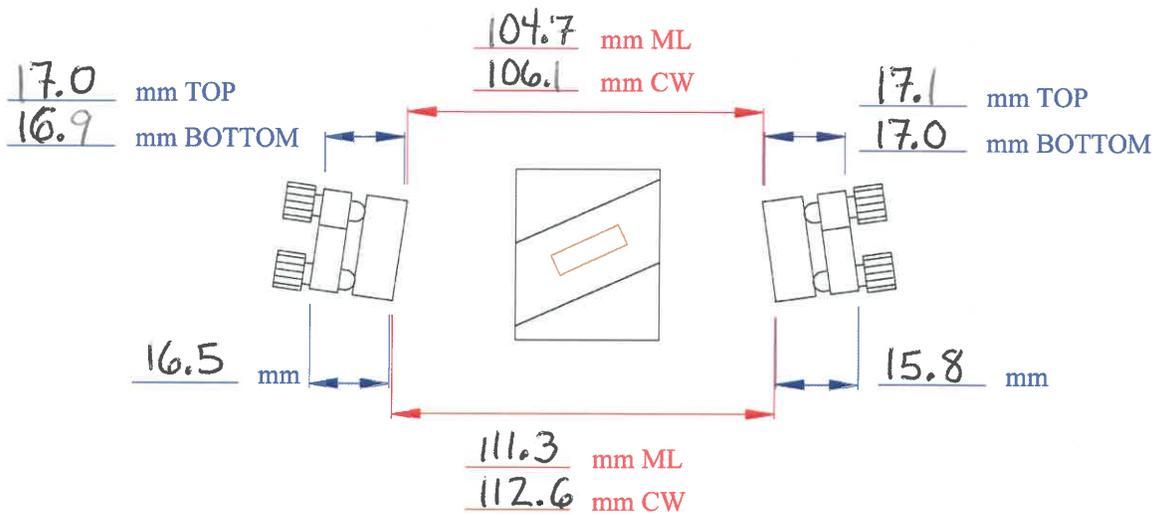
**Figure 5.6:** Detail on approximate cavity mirror adjustments to obtain the correct beam entrance/exit angles. Dimensions correspond to the thickness, measured with a caliper, between the face of the mount and the anodized aluminum base, as drawn.
