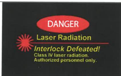
**Figure 3.2:** Interlock defeated labels (2) affixed to both sides of the entrance shutter defeat flag.
