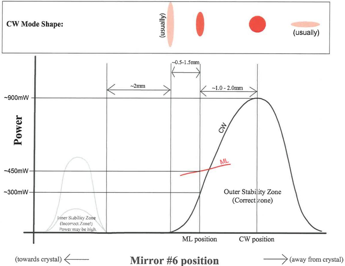
**Figure 5.7: Approximate mode shapes and power for various positions of the second curved mirror (#6). The proper position of this mirror for mode-locked operation is at the inner edge of the outer stability zone.**
