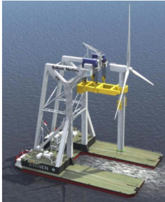
Figure 10. Turbine install concept from Ballast Nedam (2013) for the Svanen. Though not illustrative of any of the approaches discussed here, with its partial onshore assembly and vertical deployment it does share some of the same conceptual underpinnings.
