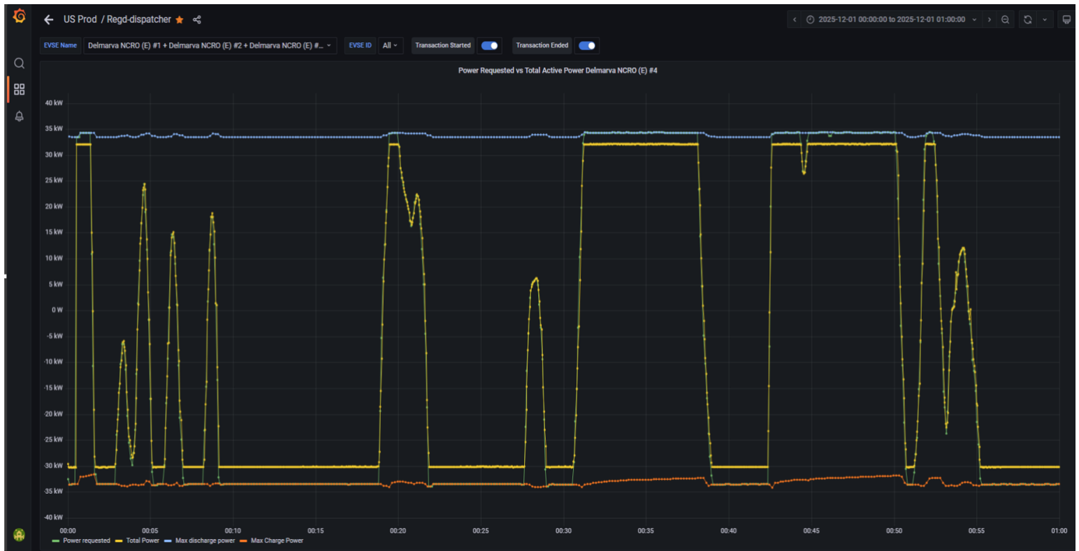
Figure 6.6. Regulation service by EV 1146 on station NCRO 4, December 1, 2025, Midnight to 1:00 am. Green is power request, yellow is metered power response. (Red is the charging maximum and blue the discharging maximum.)
