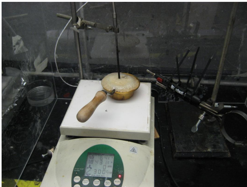
Figure 17. STF flash point experiment. Note the foam rising above the sample cup.
