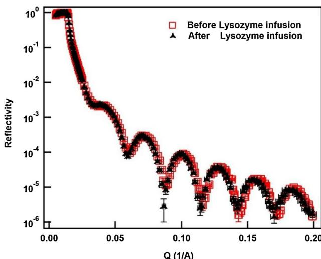
**Fig. 8.** reflectivity data of polystyrene film in D<sub>2</sub>O (red square), and after 5 mg/ml lysozyme solution is infused into flow cell (black triangle). (For interpretation of the references to colour in this figure legend, the reader is referred to the web version of this article.)
