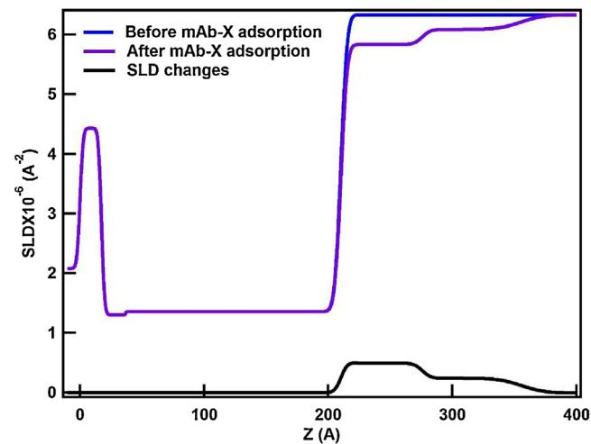
**Fig. 6.** Scattering length density(SLD) profile in  $D_2O$  before 5 mg/ml mAb-X adsorption on polystyrene film (blue line) and after 5 mg/ml mAb-X adsorption on polystyrene film (purple line). Changes in the SLD profile after 5 mg/ml mAb-X adsorption are plotted as the black line. (For interpretation of the references to colour in this figure legend, the reader is referred to the web version of this article.)
