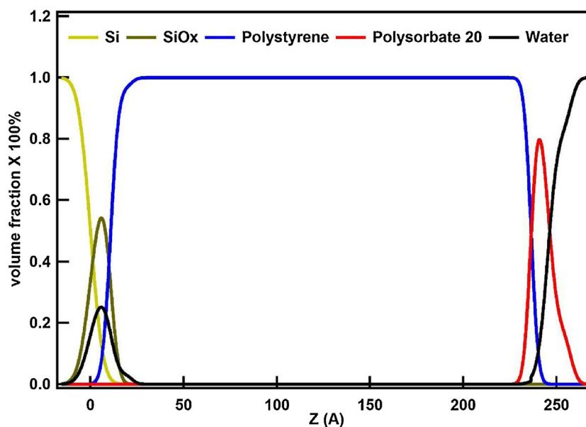
**Fig. 3.** Volume fractions of each layers after  $4.075 \times 10^{-4} M$  polysorbate 20 adsorption on polystyrene surface: silicon (gold), SiO<sub>x</sub> (brown), polystyrene (blue), polysorbate 20 (red), water (black). (For interpretation of the references to colour in this figure legend, the reader is referred to the web version of this article.)
