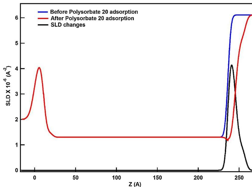
**Fig. 2.** Scattering length density (SLD) profile in  $D_2O$  before (blue line) and after (red line)  $4.075 \times 10^{-4} M$  polysorbate 20 adsorption on polystyrene film. Changes in the SLD profile after  $4.075 \times 10^{-4} M$  polysorbate 20 adsorption is plotted as the black line. (For interpretation of the references to colour in this figure legend, the reader is referred to the web version of this article.)
