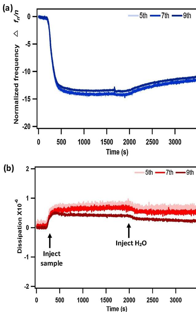
**Fig. 4.** (a): normalized frequency changes of each overtone after  $4.075 \times 10^{-5}$  M polysorbate 20 is infused into flow cell and (b): corresponding dissipation value of each overtone.
