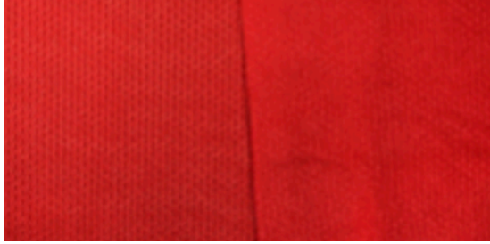
Right (Front) Wrong (Back) *The wrong side does not contain obvious meshes
