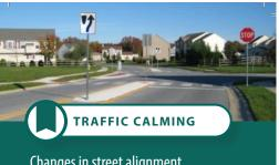
Changes in street alignment, installation of barriers, and other physical measures to reduce traffic speeds or cut-through volumes, in the interest of street safety and livability.
