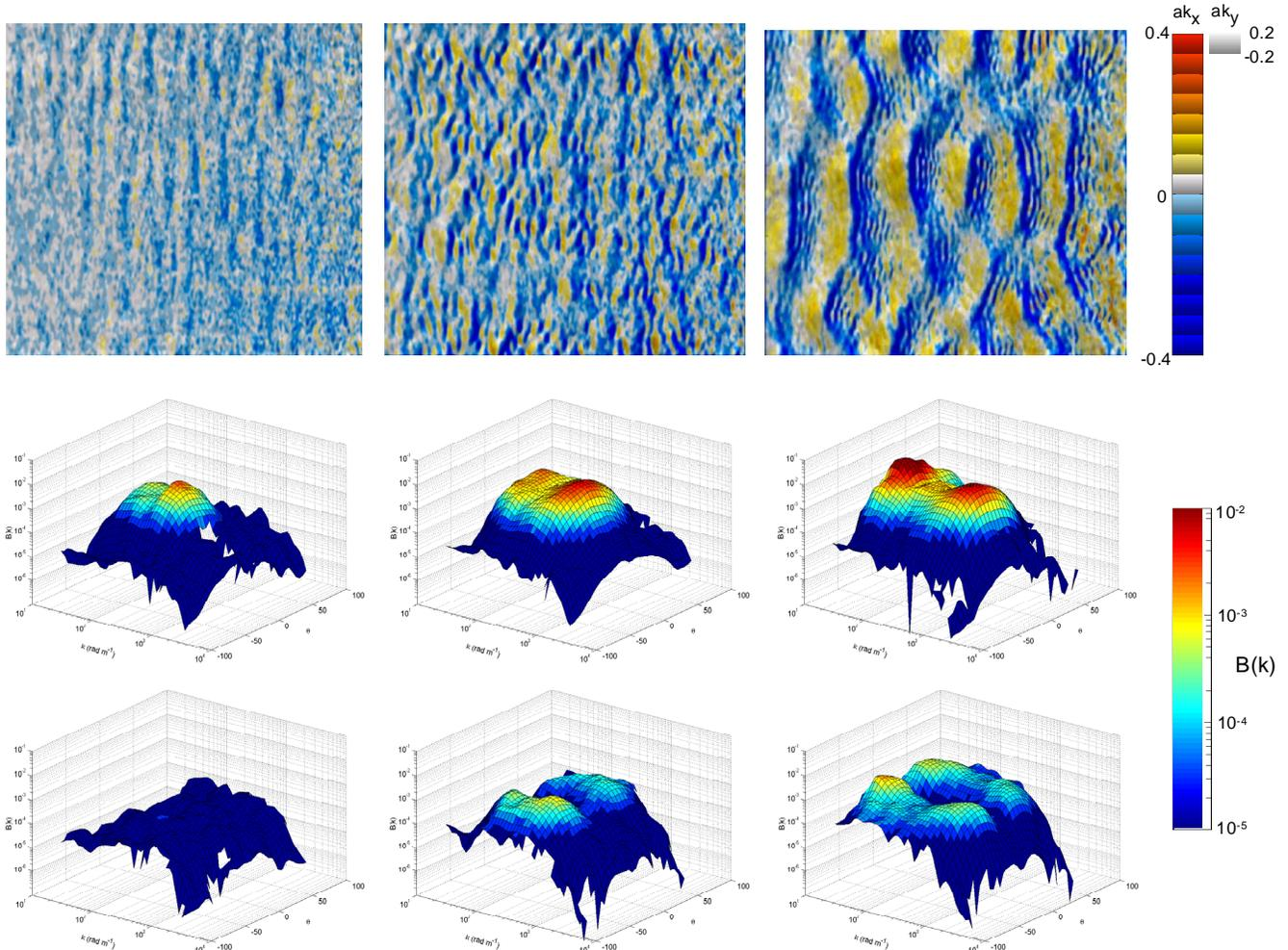
Fig. 2 Surface slope images for a final wind speed of  $5\text{ms}^{-1}$  Image size is  $26.5 \times 36 \text{ cm}$ . Time shown are  $t=15, 25,$  and  $35\text{s}$ . The color code shows the along-wind slope and the shading corresponds to the cross-wind slope. Below each slope image is the corresponding directional saturation spectrum for the along-wind slope and cross-wind slope respectively.
