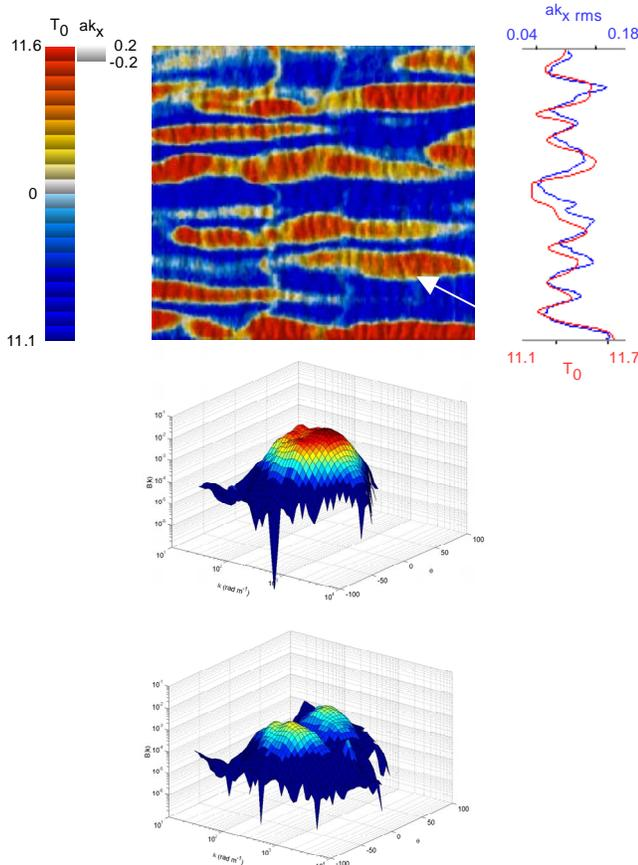
Fig. 3 Co-located surface temperature (color) and wave slope (shading) at  $t=19.8$  s for a final wind speed of  $5 \text{ ms}^{-1}$ . The surface temperature (modulated by the sub-surface velocity) is clearly coupled with the surface waves which consequently develop slopes in the cross-wind direction as shown in the spectra.
