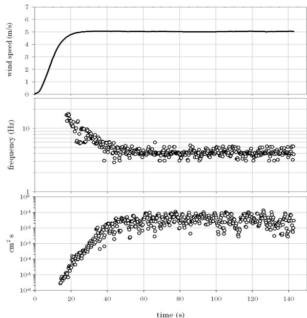
Fig. 1 Wind speed, peak frequency and peak power density of the wave field as a function of time.
