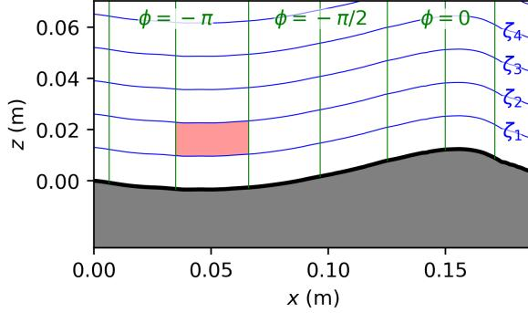
FIG. 2. Plot of the coordinate system used in the analysis. The green lines indicate a constant phase ( $\phi$ ), as detected using the Hilbert transform method. The blue lines indicate lines of constant  $\zeta$  and the black line is the water surface ( $\zeta = 0$ ). The red region exemplifies a bin as used in the phase averaging process, albeit much bigger than those actually used. All values within the same bin are averaged together.
