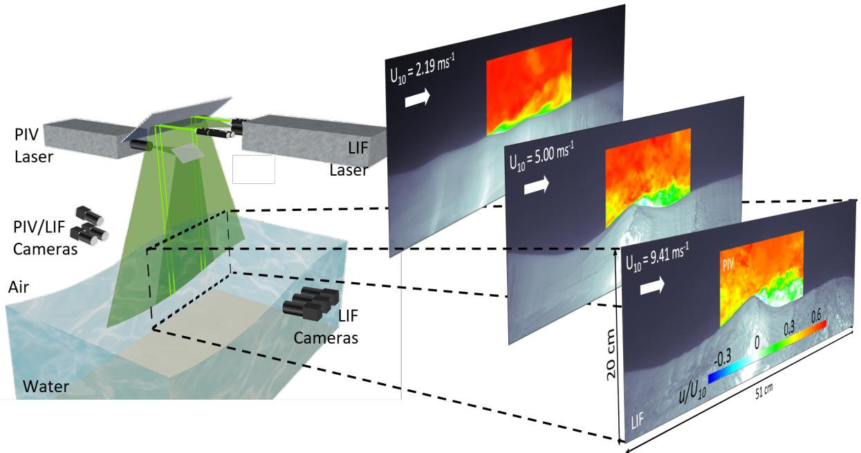
FIG. 1. Sketch of the experimental setup, placed at a fetch (i.e., distance down-wind from the onset of wind-wave growth) of 22.7 m within University of Delaware’s large wind-wave-current facility, along with examples of composite instantaneous two-dimensional LIF-PIV data products, for the three wind speeds examined here ( $U_{10} = 2.2, 5.0, \text{ and } 9.4 \text{ m s}^{-1}$ ).
