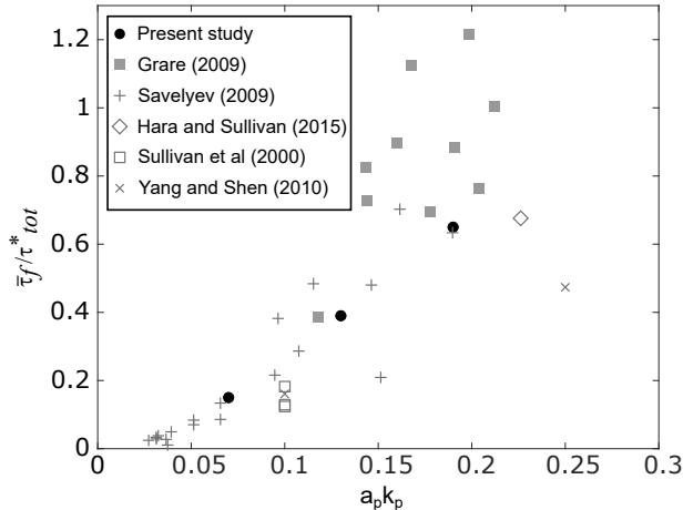
FIG. 5. Mean normalized form drag estimated using 2D pressure fields retrieved from 2D airflow PIV measurements over laboratory wind waves, normalized by the total stress, plotted versus wave slope (black symbols). Results from pressure measurements above mechanically generated waves from previous laboratory studies (Grare 2009; Savelyev 2009) are also shown, as well as previous form drag estimates from LES (Hara and Sullivan 2015) and DNS (Sullivan et al. 2000; Yang and Shen 2010).
