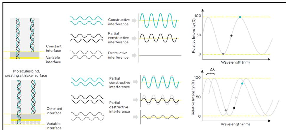
**Figure 1B: Principle of biolayer interferometry**
