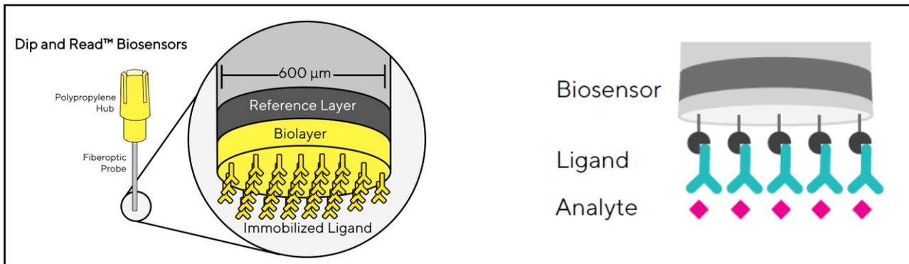
**Figure 1A: Biolayer sensor tip**
