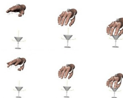
Fig. 7. On the top figure snapshots of the trajectory conducted by the human during grasping a glass are depicted. On the bottom figure snapshots of the simulated hand following the trajectory generated by the proposed control law during grasping a glass are depicted. In this figure the side view of the grasping experiments is depicted.
