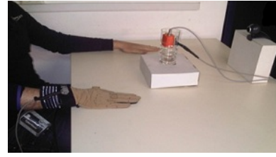
Fig. 1. A human subject before the initiation of a reach to grasp movement. The two position trackers are placed on the user's wrist joint and on the object. The human hand kinematics are captured with CyberGlove 2 motion capture glove and the IMU is placed inside the object.
