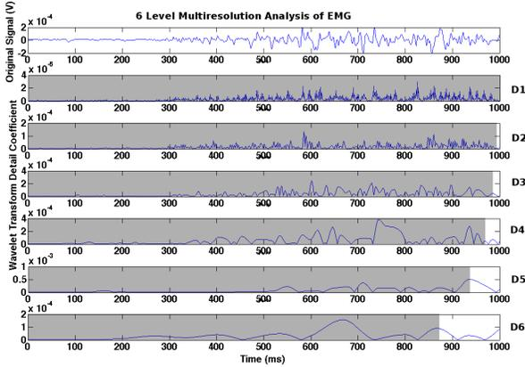
Figure 2. Example 1D 6 level DWT. The top plot shows the original signal, and each consecutive plot below shows the detail coefficients  $D_n$  resulting from the wavelet transform at level  $n$ . The shaded region represents discarded coefficients when extracting features at time 1000ms.
