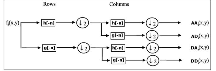
Figure 1. The 1 Level 2D wavelet transform.
