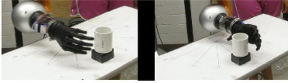
Fig. 3. Hand configuration in testing phase. Left: normal configuration from learning phase. Right: rotated configuration.
