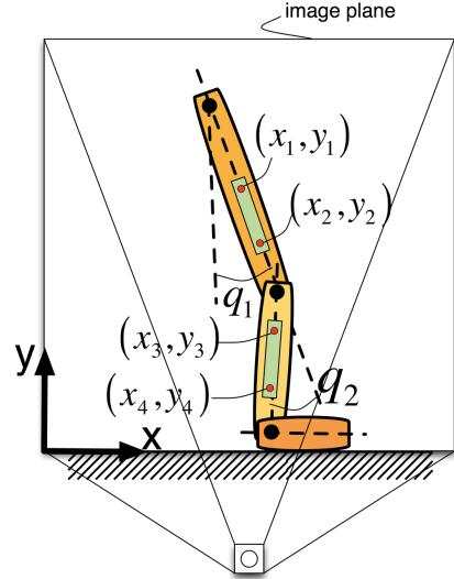
Figure 2. The computation of hip flexion-extension ( $q_1$ ) and knee flexion-extension ( $q_2$ ) is done using the coordinates of each LED at the image plane reference system, included in the LED modules. Offset values of joint angles are discarded through an initial calibration procedure.
