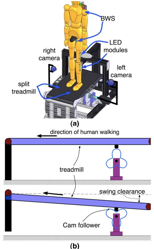
Figure 1. (a). The MIT-Skywalker platform used for the perturbation experiments. The subject's weight is supported by the body-weight support (BWS) including a saddle-like seat and a chest harness. Two cameras and four LED modules were used for leg motion tracking. (b). Cam-based mechanism of the vertical actuation of the treadmill. As the cam rotates, the follower comes into the low dwell of the cam and a swing clearance of 8.9 cm is created.
