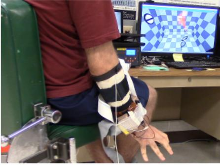
Fig. 2. VR control setup including the sEMG systems and monitor.
