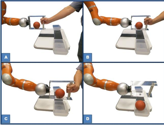
Fig. 2. Process of Trial: A) Initial start of trial, B) Beginning of lateral movement, C) End position at bin, D) Rotation by robot and ball drop into bin.
