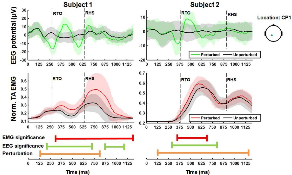
Fig. 3: EEG potential at the CP1 location and normalized EMG for the tibialis anterior (TA) for both subjects. Mean (darker lines) and standard deviations (lightly shaded areas) values are shown for the perturbed and unperturbed gait cycles. Statistically significant changes are indicated by colored bars that correspond to the type of neural signal. An indication of the timing of the perturbation is also shown. RTO and RHS correspond to toe-off and heel-strike of the right leg, respectively.
