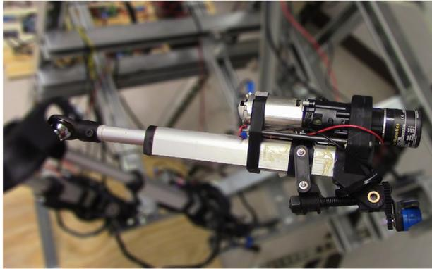
**Fig. 5 Motion coupled actuator. Conceptual model (top) with the following components: (A) motor, (B) custom gearbox, (C) pitch/stroke encoder, (D) roll measurement potentiometer, (E) wormscrew, (F) pitch/stroke coupling linkage, (G) pitch control slider, (H) enclosed limit switches, (I) tie rod joint, and (J) enclosed powerscrew and slider for linear actuation. Developed prototype (bottom).**
