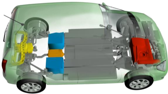
Fig. 2. HEV configuration showing the engine (red), the inverter (orange), the battery packages (blue), and the electric machines (yellow).
