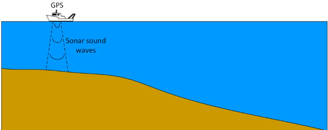
Figure 11. Schematic showing a survey vessel with GPS and sonar device for offshore beach profile measurements.
