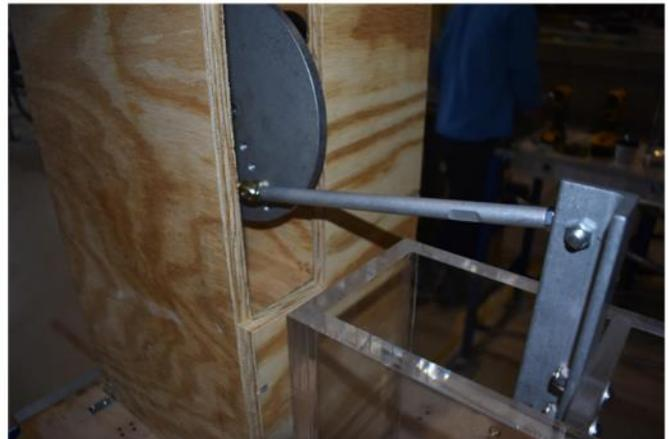
Figure A13. Pictures showing attachment of linkage arm to wave flume paddle arm.
