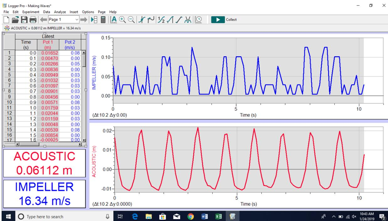
Figure A29. LoggerPro screenshot showing highlighting of sensor data for copying into an Excel spreadsheet.
