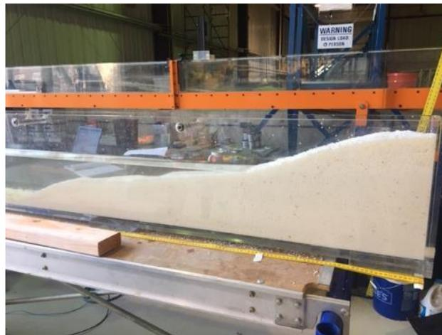
Figure A15. Initial beach set up in a roughly triangular shape.
