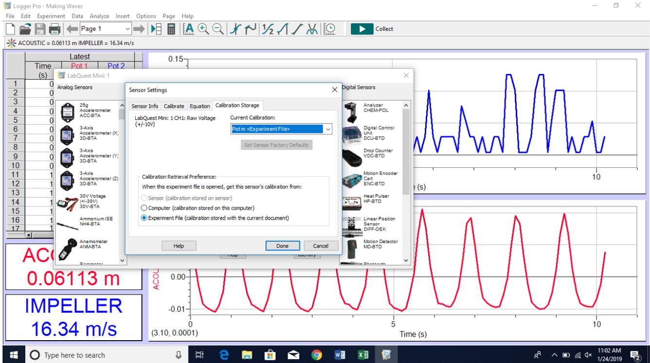
Figure A32. LoggerPro screenshot showing options for setting up sensors – calibration storage (ONLY IF NEEDED).
