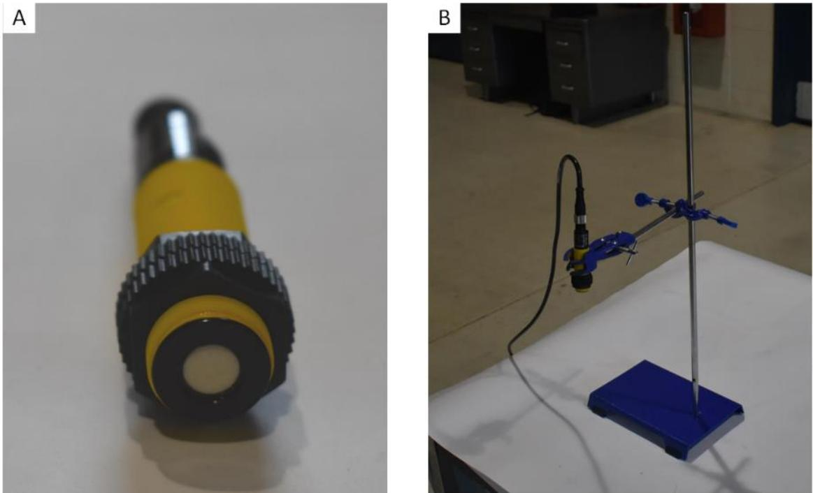
Figure A23. A) The Banner Acoustic Distance Meter. B) The acoustic sensor in the lab stand.
