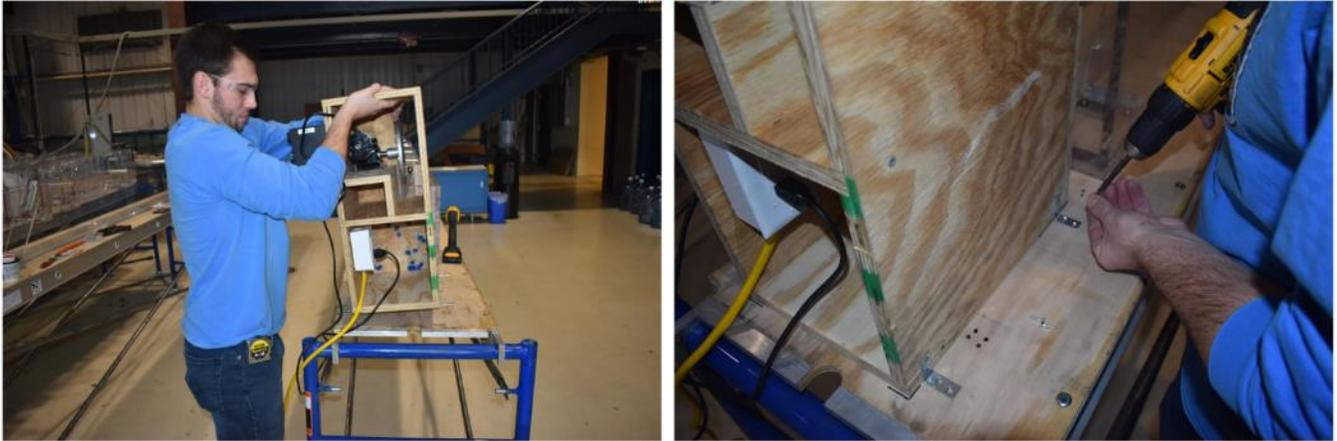
*Figure A12. Pictures showing motor assembly stand and stand placement on scaffold plank.*
