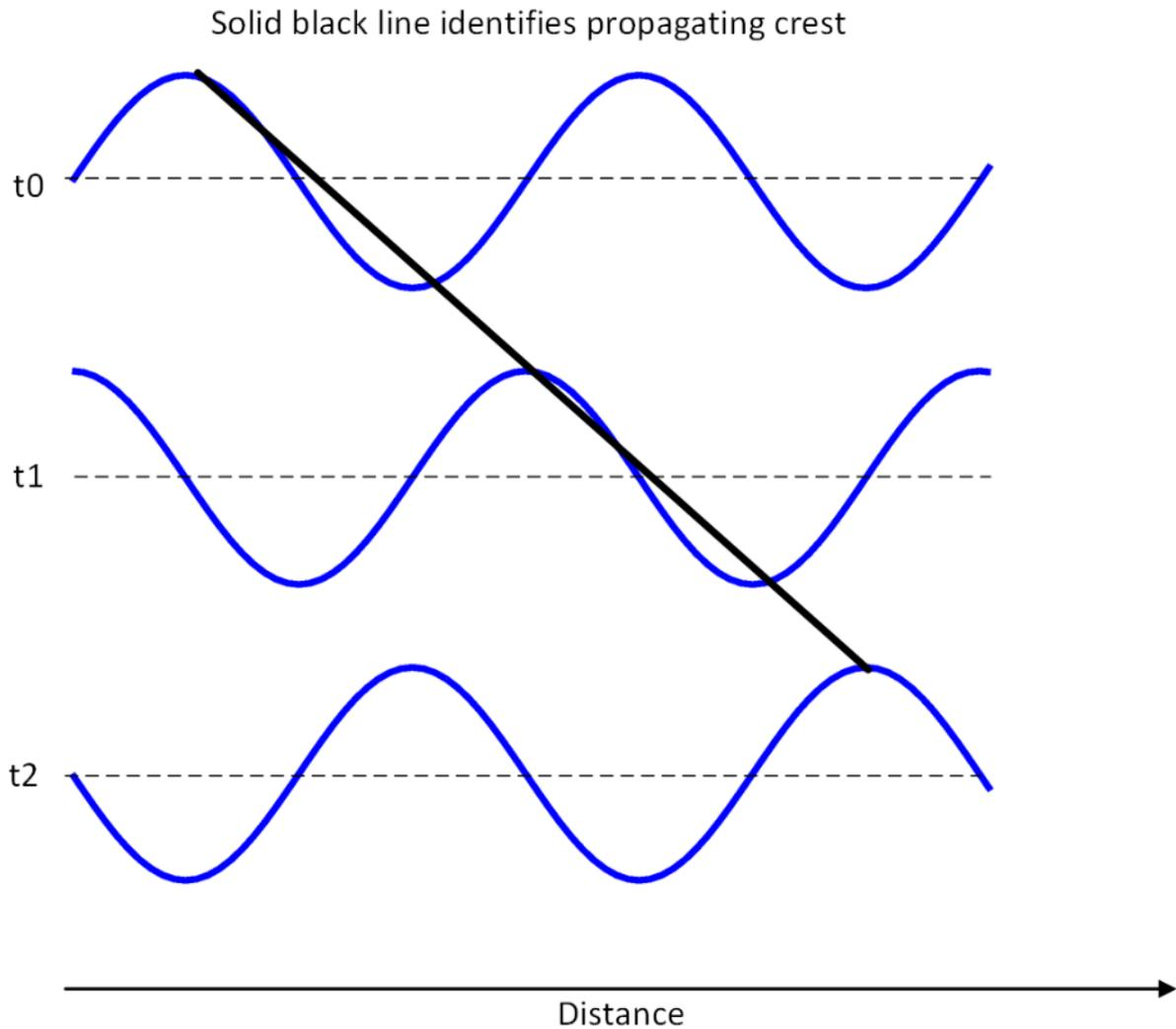
Figure 6. Schematic showing the propagation of a wave crest
