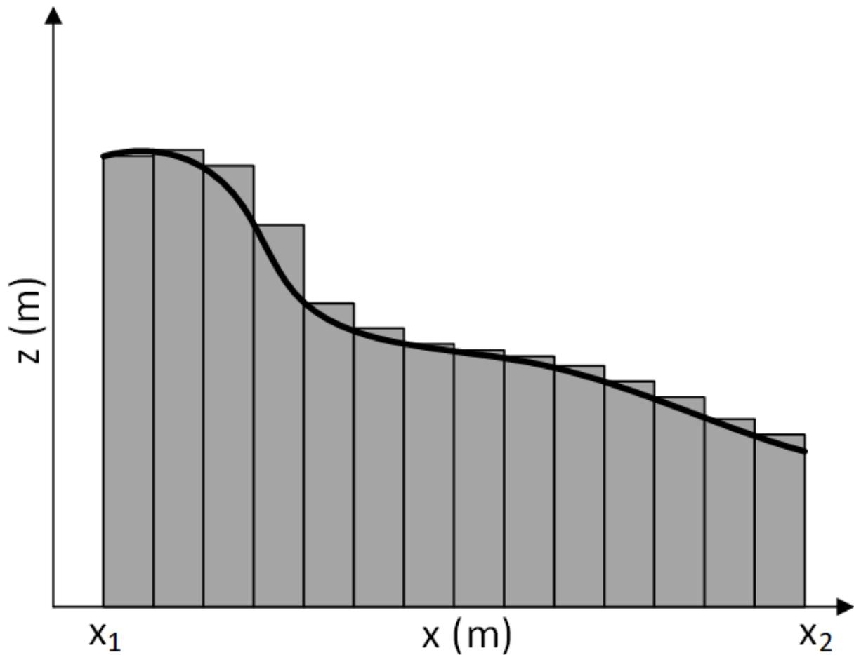
Figure 18. Schematic showing the left-point rule for integration for area under the curve.
