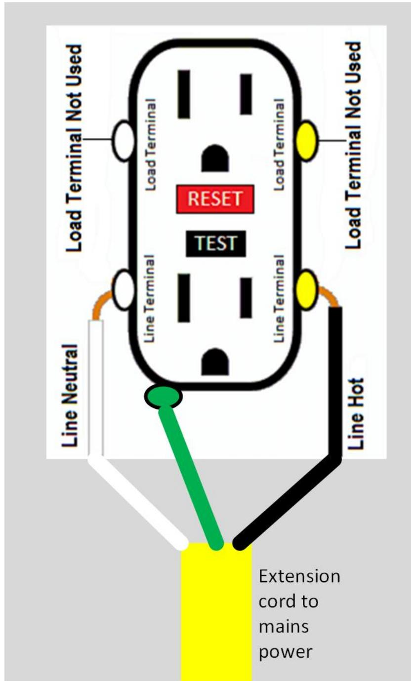
Figure A38. Wiring diagram for the GFCI outlet for the wave flume motor assembly stand.
