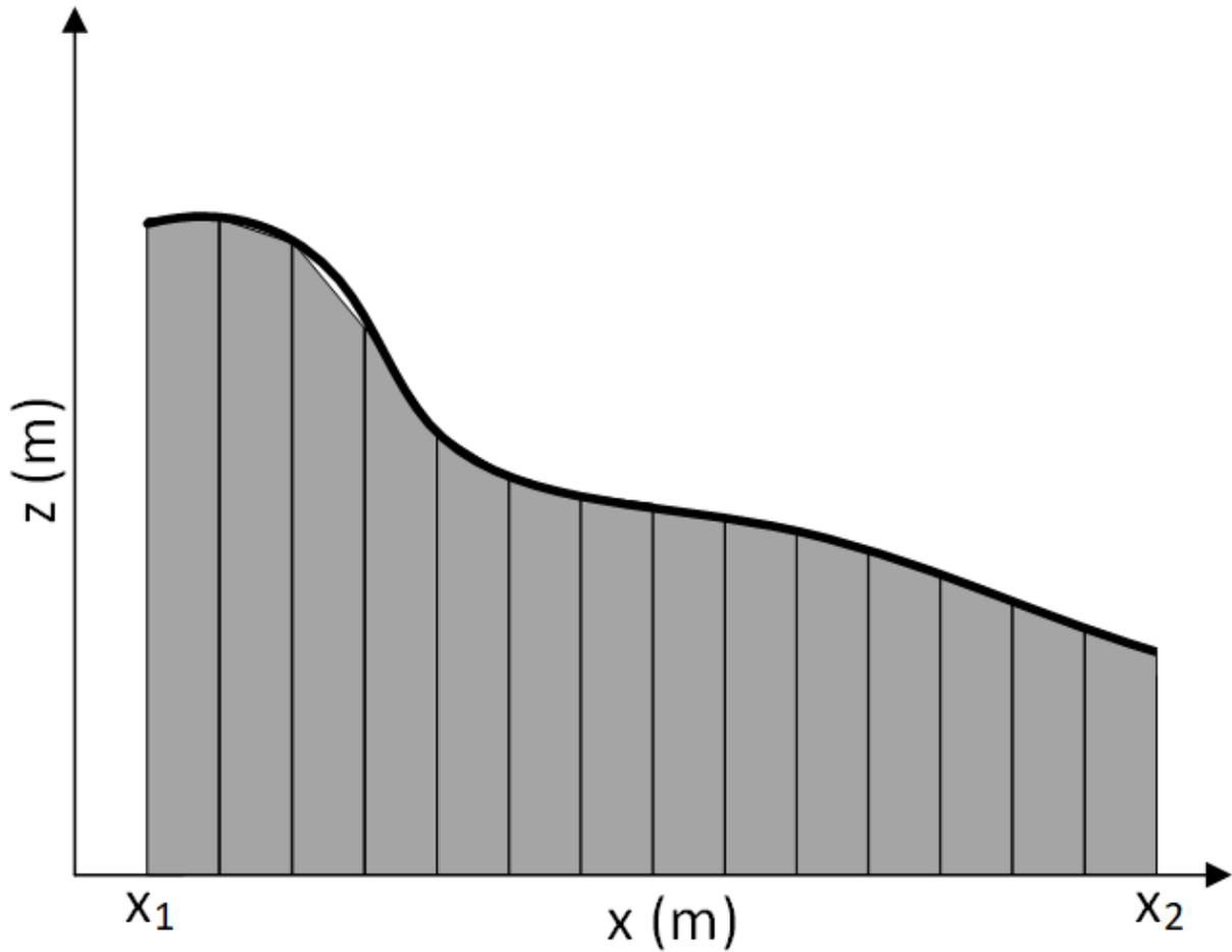
Figure 19. Schematic showing the trapezoid rule for integration for area under the curve.
