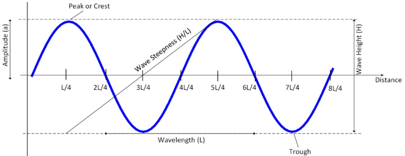
Figure 3. Image showing the parts and parameters of a wave train.
