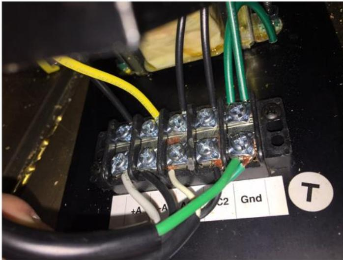
Figure A37. Wiring diagram and picture showing the wiring inside the DC speed controller.
