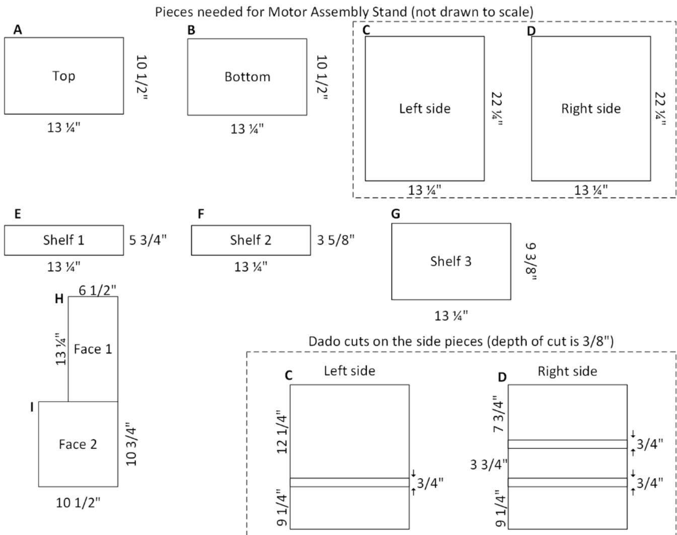
Figure A35. Diagram showing pieces, dimensions, and dado cuts for motor stand assembly. Letters correspond to pieces of completed stand shown in Figure A36.
