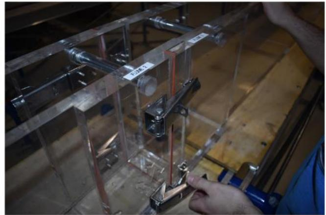
Figure A9. Pictures showing mating of flume halves and adjustment and closing of draw latches.
