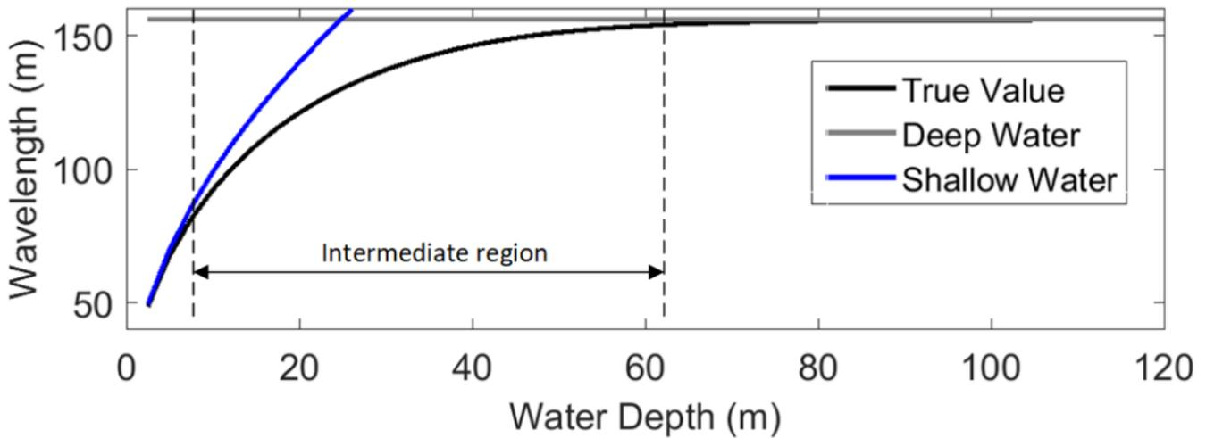
Figure 4. Wavelength as a function of water depth with deep and shallow water estimates shown in relation to the true wavelength.
