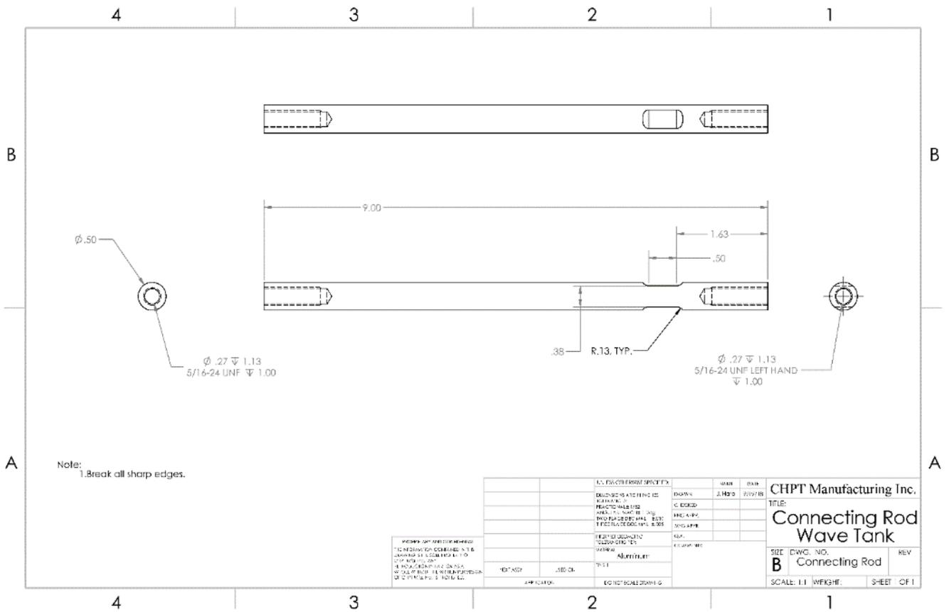
Figure A20. Snapshot of CAD drawing for the linkage arm. A PDF version of the file is available upon request.
