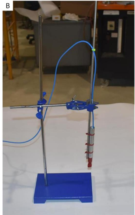
Figure A24. A) Close up view of the Omni Instruments Impeller Current Meter. B) The impeller attached via cable ties to a  $\frac{1}{4}$ " diameter stainless steel tube and affixed in the lab stand.
