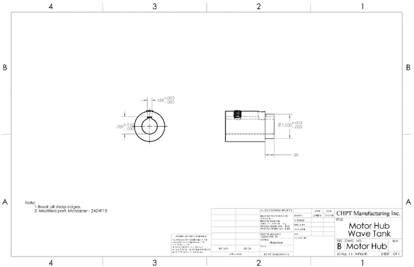
Figure A21. Snapshot of CAD drawing for the motor hub. A PDF version of the file is available upon request.
