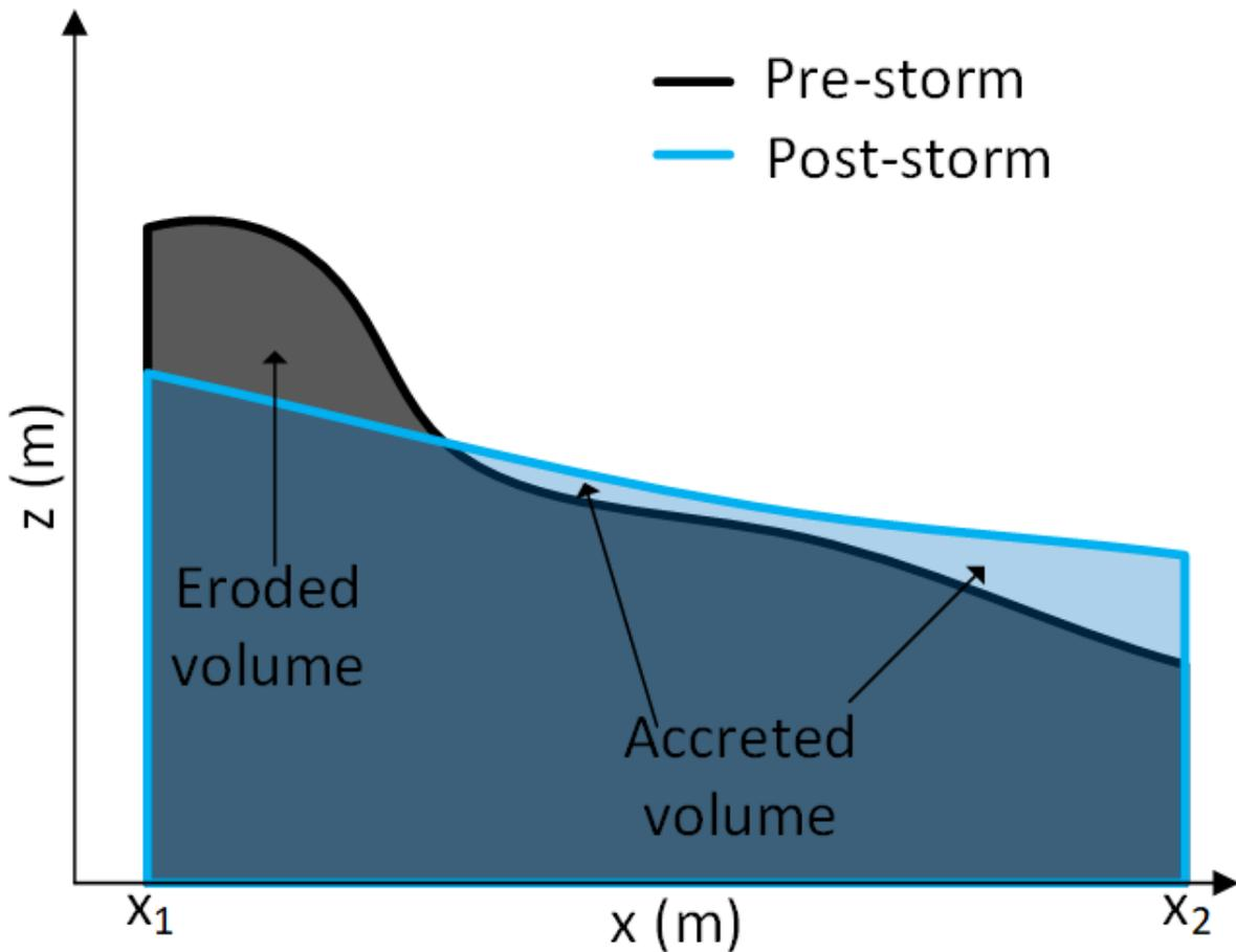
Figure 17. Schematic showing the areas under the curve determined through integration and eroded and accreted volumes from pre- and post-storm measurements.
