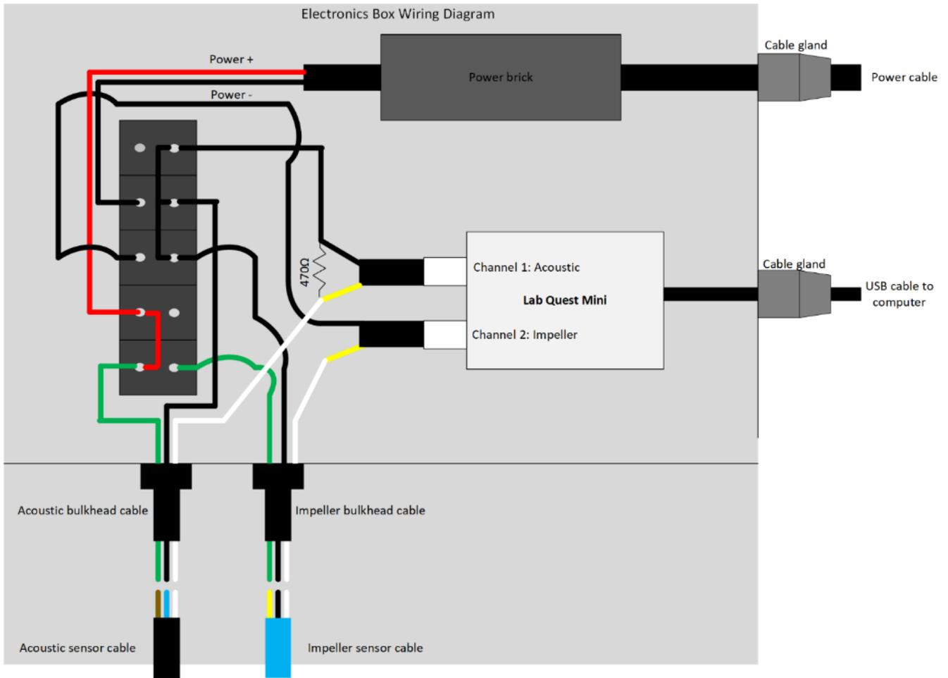
Figure A34. A wiring diagram for the electronics box.
