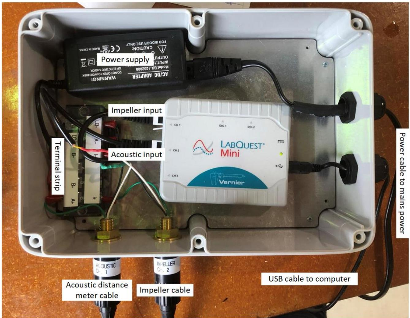
Figure A33. A picture of the electronics box showing the main components.
