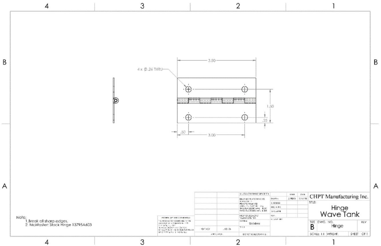
Figure A22. Snapshot of CAD drawing for the hinge connecting the wave paddle to the flume. A PDF version of the file is available upon request.
