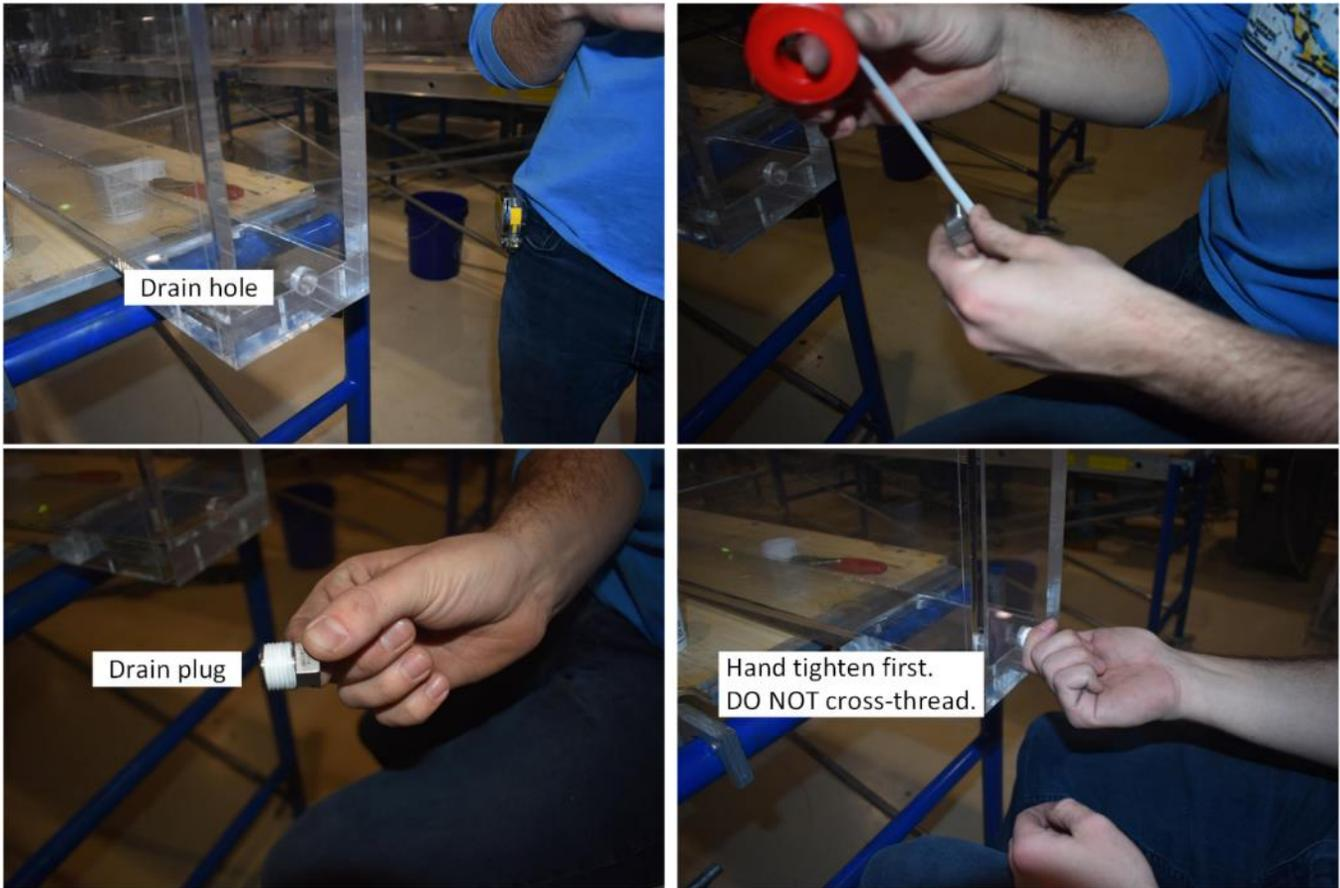
Figure A11. Pictures showing drain hole and drain plug.
