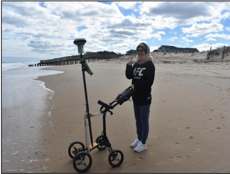
Figure 10. Student surveying a beach profile using a low-cost push cart and high grade GPS equipment. The antenna is at the top of the pole.
