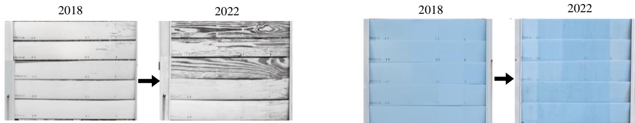
Figure 1. Images of panels displaying cracking & checking (left) and discoloration (right) [Images provided by Arkema]
