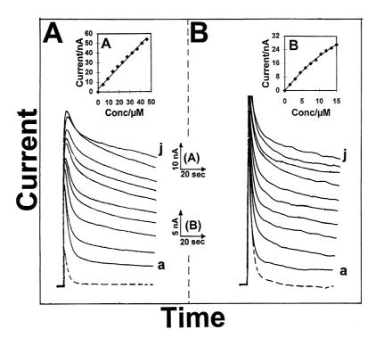
Fig. 1. Chronoamperometric response to an untreated river water sample containing increasing levels of paraoxon (A) and methyl parathion (B) in  $4.6 \times 10^{-6}$  M and  $1.5 \times 10^{-6}$  M steps, respectively (a–j). Dotted lines represent the response of the unspiked samples. Potential step to +0.85 V.
