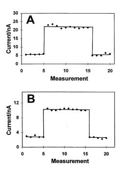
Fig. 2. Carry over experiments. Untreated river water samples, containing  $4.6\times10^{-6}\,\mathrm{M}$  and  $23.0\times10^{-6}\,\mathrm{M}$  paraoxon (A) or  $1.5\times10^{-6}\,\mathrm{M}$  and  $7.5\times10^{-6}\,\mathrm{M}$  methyl parathion (B). Other conditions, as in Figure 1.
