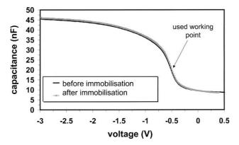
Fig. 3. Capacitance/voltage (C/V) curve of a capacitive field-effect sensor with  $Si_3N_4$  as pH-sensitive material before (full line) and after enzyme immobilization (open squares) via glutaraldehyde.
