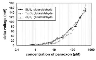
Fig. 7. Influence of the calibration plot towards paraoxon of the enzyme biosensor on the pH-transducing layer used (Si<sub>3</sub>N<sub>4</sub>, Al<sub>2</sub>O<sub>3</sub> and Ta<sub>2</sub>O<sub>5</sub>). Each data point represents the mean value of three measuring points for paraoxon concentrations above 15  $\mu M$ , and the mean value of five measuring points of concentrations below 15  $\mu M$ . The error bars represent  $\pm 1$  standard deviation.
