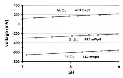
Fig. 4. The pH sensitivity of the EIS biosensor after enzyme immobilization. Al<sub>2</sub>O<sub>3</sub>, Ta<sub>2</sub>O<sub>5</sub> and Si<sub>3</sub>N<sub>4</sub> serve as transducer materials.
