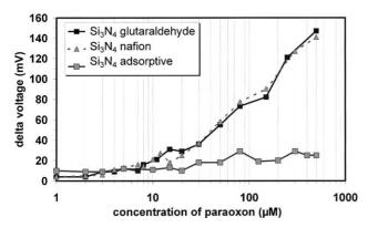
Fig. 6. Calibration curve of the enzyme biosensor for paraoxon with  $\mathrm{Si}_3\mathrm{N}_4$  as pH-sensitive transducer. The enzyme OPH was immobilised by adsorptive-, nafion- and glutaraldehyde coupling.
