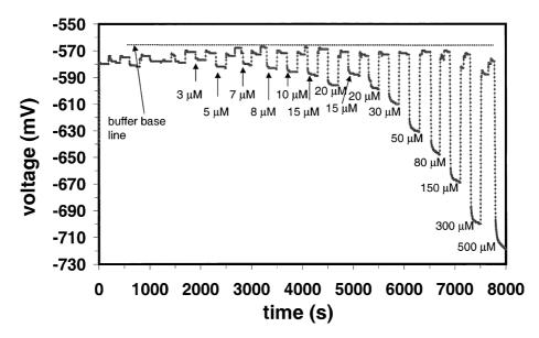
Fig. 5. Typical constant capacitance (ConCap) plot vs. time of the EIS biosensor. The dotted line corresponds to the buffer concentration that is alternatingly measured with the increasing paraoxon concentration.
