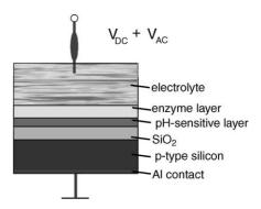
Fig. 1. Capacitive EIS biosensor with immobilised enzyme layer on a pH-sensitive transducer structure (schematically).
