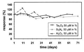
Fig. 8. Comparison of the long-term stability of the three different enzyme biosensors with the transducer materials  $Si_3N_4$ ,  $Al_2O_3$  and  $Ta_2O_5$ . For each sensor, the first measurement was defined as 100% response.
