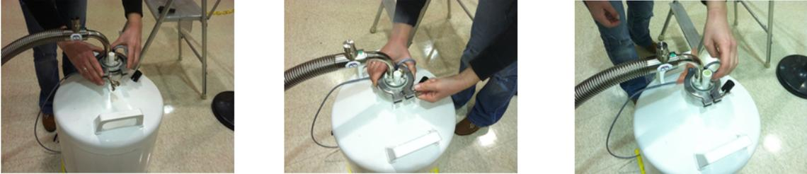
**Figure 14: Screw down the Seal Clamp and the Green Cap**
