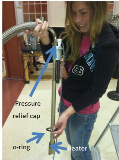
**Figure 12: The o-ring and Pressure Relief Cap**
