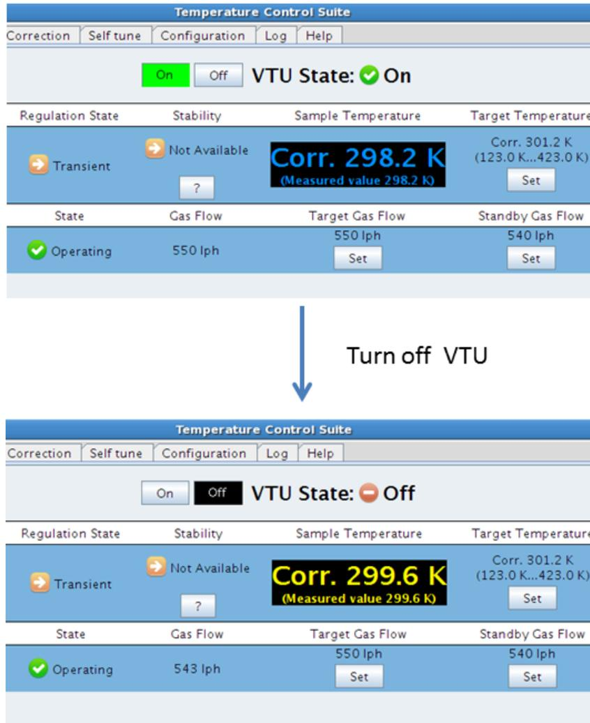
**Figure 10: Turn Off the Variable Temperature Unit**
