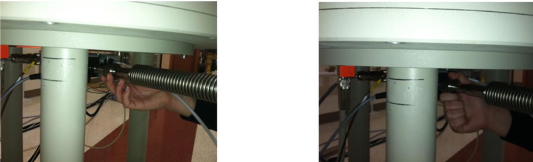
**Figure 15: Insertion of the Transfer Line into the Probe**
