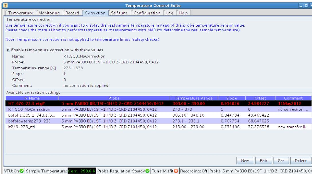
Figure 3: Select Appropriate Temperature Correction Parameter File
