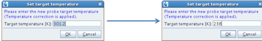
**Figure 20: Set a Target Low Temperature**
