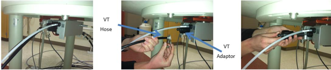
**Figure 11: Remove the VT Gas Hose and the VT Adaptor from Probe**
