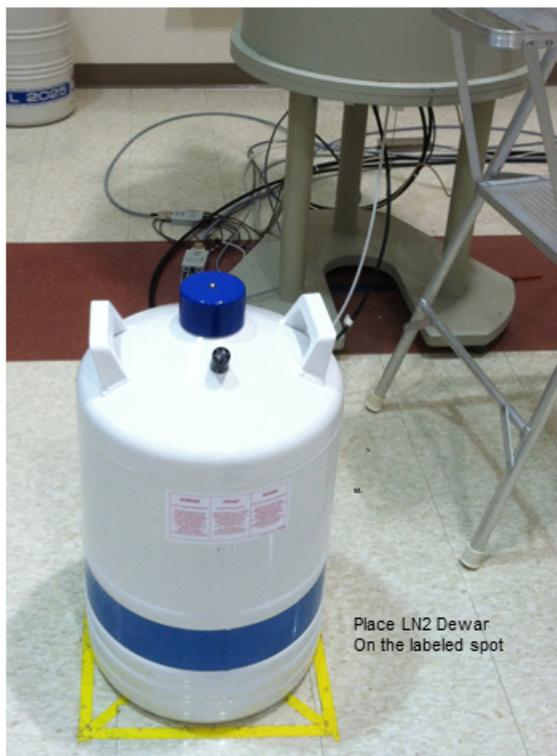
**Figure 8: Liquid Nitrogen Dewar on Labeled Spot Near the Magnet**
