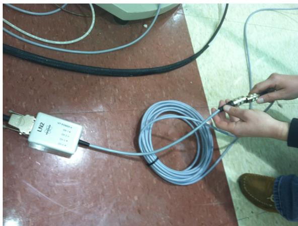
Figure 16: Connecting Transfer Line Cable to the LN2 Box
