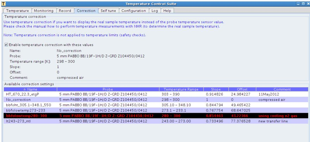
**Figure 18: Selection of Correction Parameter Settings**
