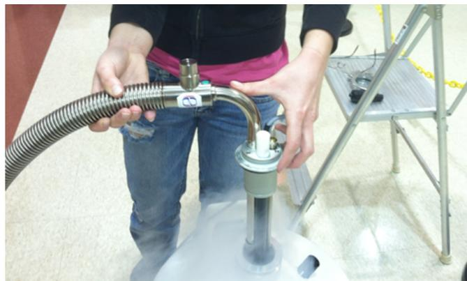
**Figure 13: Insertion of N2 Transfer Line into LN2 Dewar**
