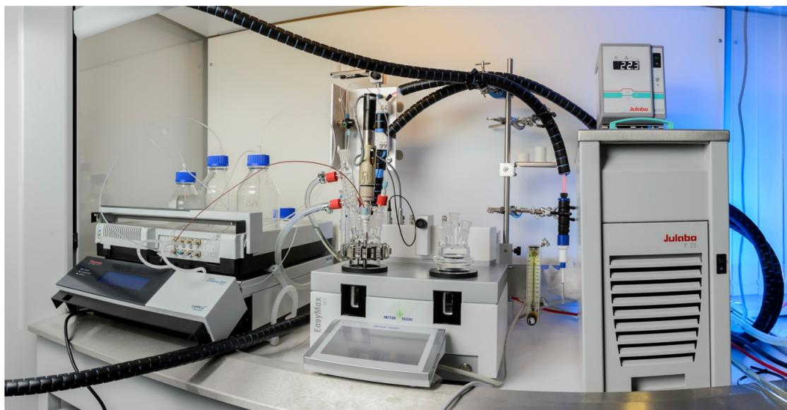
Figure 6.3: The InsightMR Flow Unit. From left to right: the pump, the reactor, the flow tube assembly secured with a clamp stand and the thermostat.
