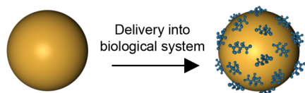
Figure 2. Gold nanoparticles delivered into biological systems are rapidly coated with proteins, which stabilize the AuNPs to prevent aggregation. AuNP binding also alters protein conformation to inhibit protein function.
