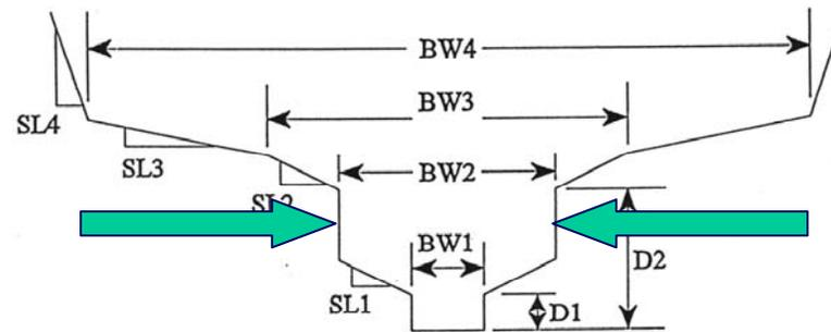
D1 = Low flow inner channel depth (ft, m)
