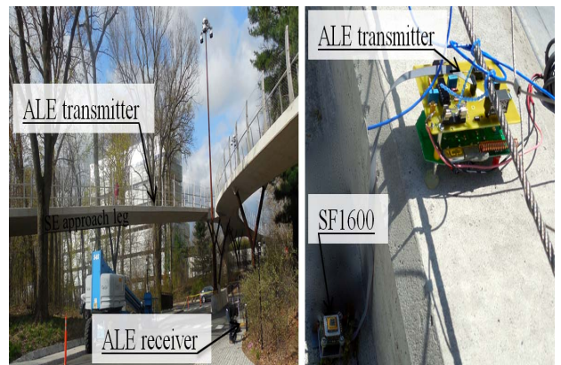
Fig. 5. Test setup and ALE deployment on the bridge
