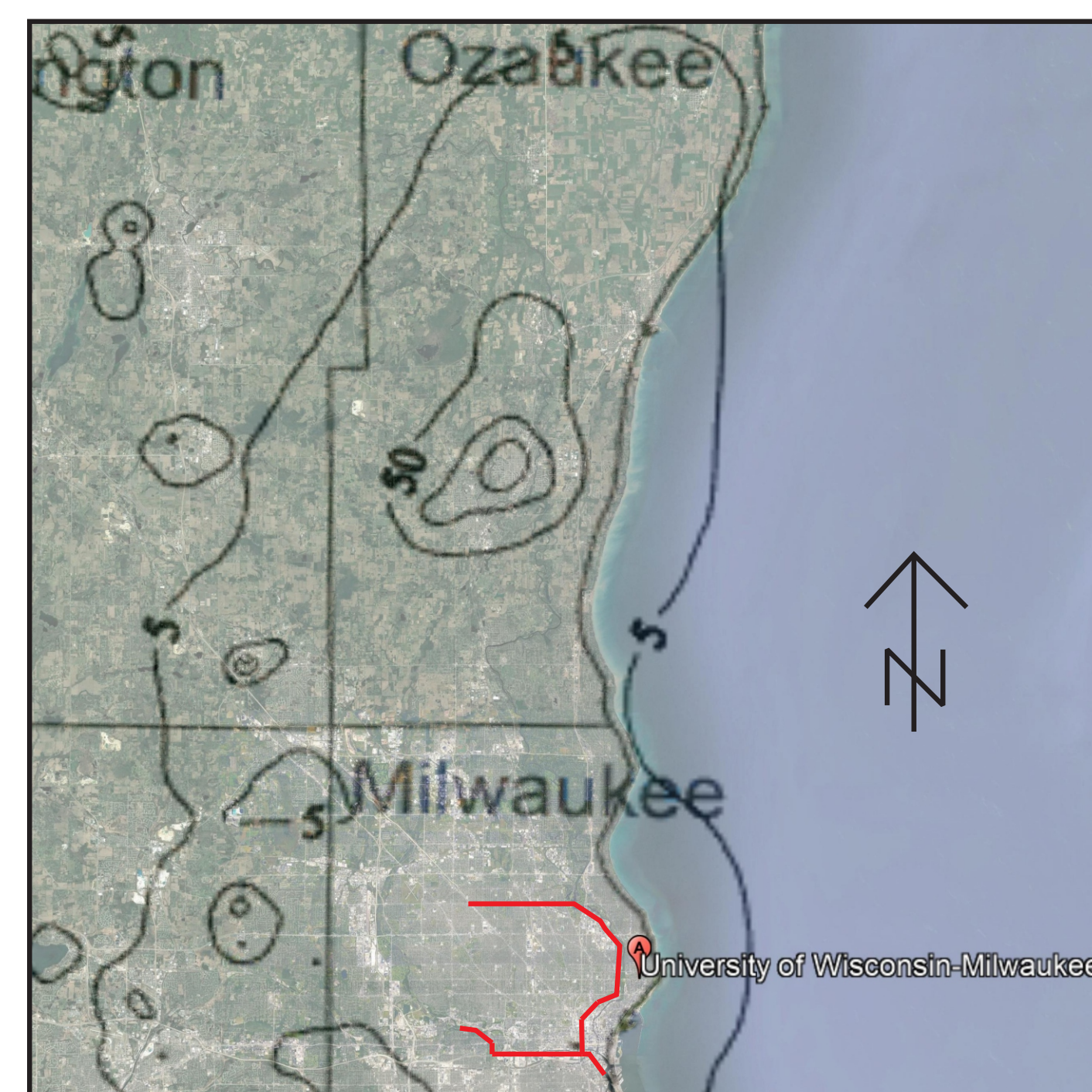
Figure 1. Regional drawdown (black contours) and approximate location of deep tunnel system (red line) relative to UWM.
