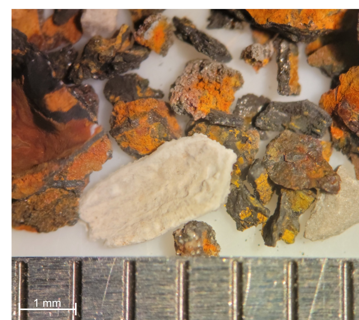
Figure 6. 10x view of material recovered from 500 \mu\text{m} screen. Scale in 1mm increments.
