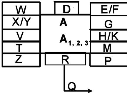
Figure 5-1. Friendly and Neutral Ground Equipment Labeling Fields
