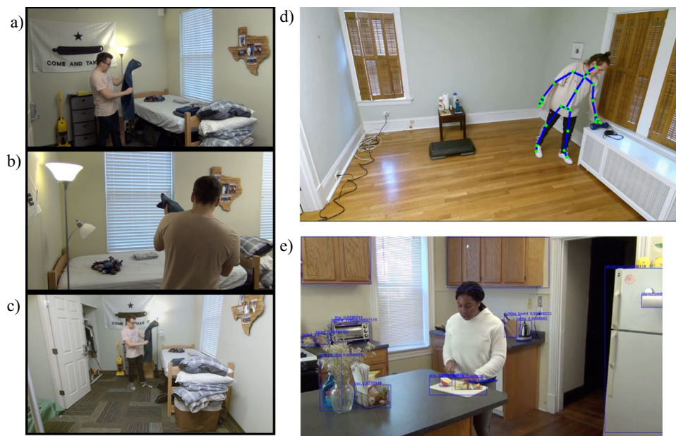
Fig. 2 Examples of performance capture and annotations. Each chapter was captured from (a, b) two HD color cameras and (c) a Kinect v2 camera. d) Skeleton joint positions were estimated in three-dimensional space and mapped to the two-dimensional Kinect color
