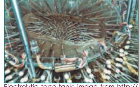
Electrolytic torso tank; image from http://www.sci.utah.edu/research/forward-sim.
