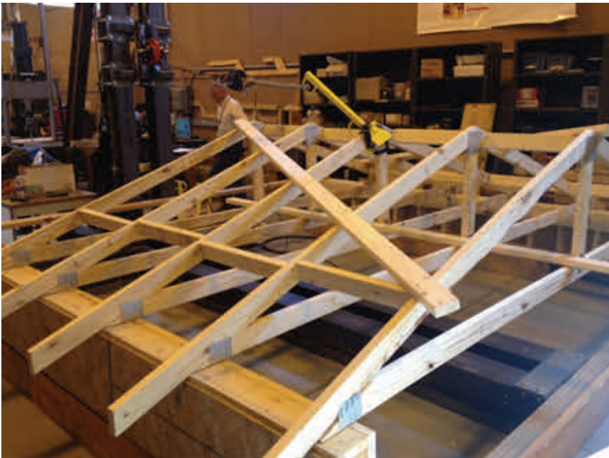
Figure 10. Five Truss System with Blocking Showing Bracing Pullout Near PFAS
