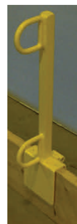
Figure 3. PFAS Anchor Used for Testing
