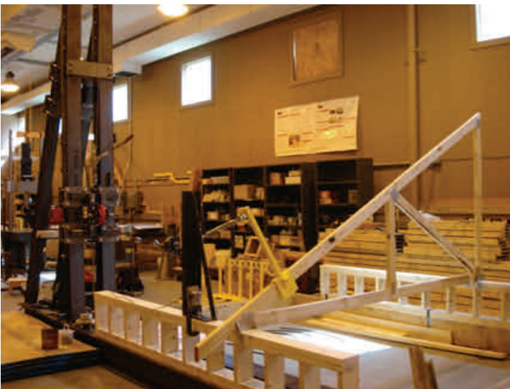
Figure 4. Testing of Monoslope Trusses Using HALT
