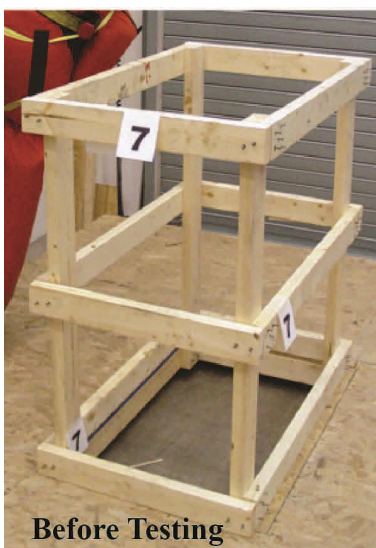
Figure 3. Subject #7 PTF Testing Results Using Nail Fasteners
