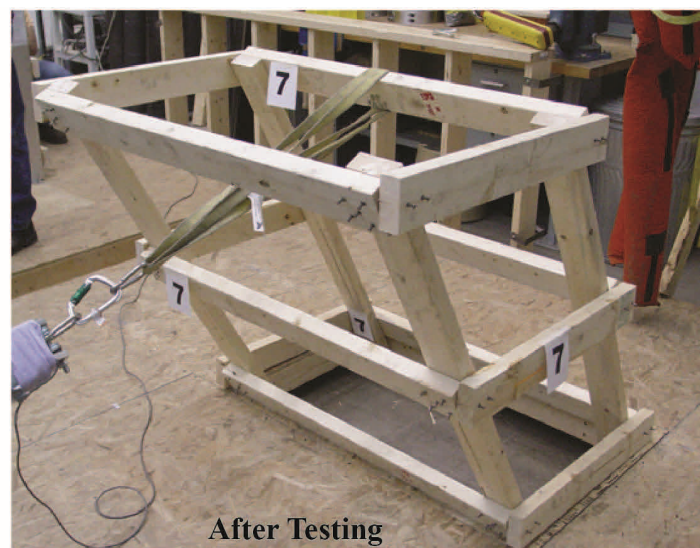
Figure 3. Subject #7 PTF Testing Results Using Nail Fasteners
