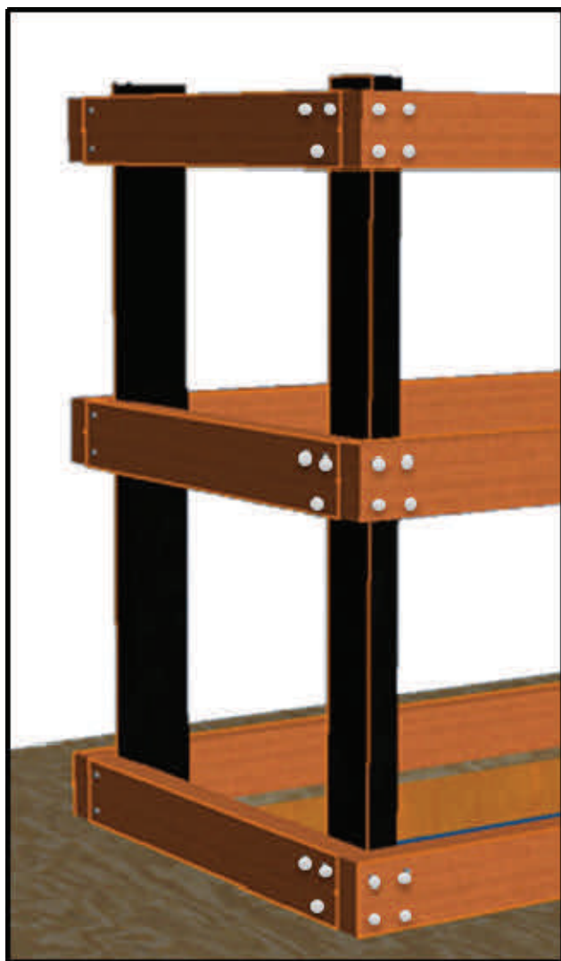
Figure 11. Overlapped Rails and Fastener Placement
