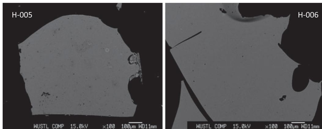
**Figure 1.** Backscattered electron (BSE) images of silicate glasses H-005 and H-006.
