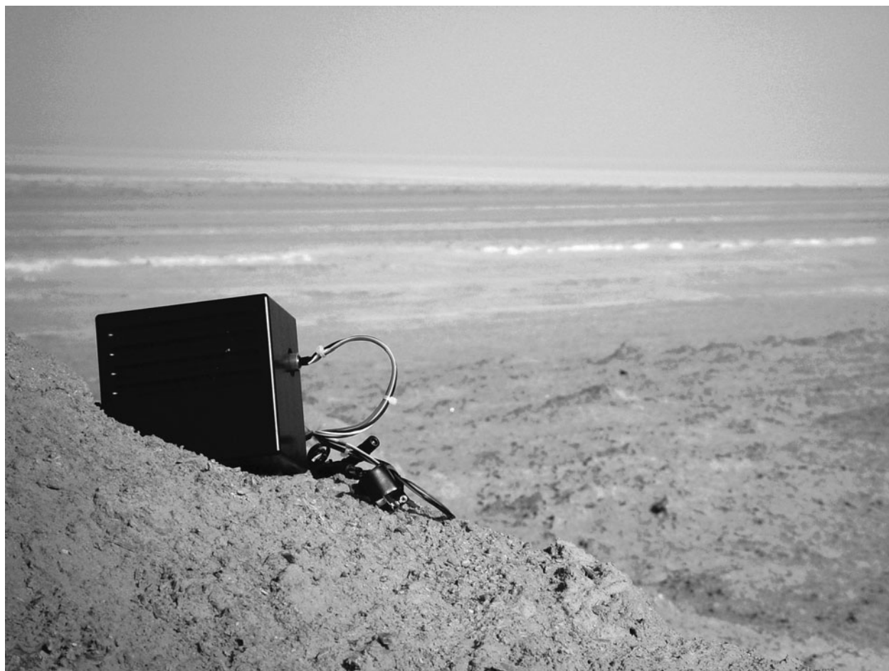
FIG. 5. WIR II instrument recording in situ NIR spectra at the Xiaoliangshan anticline in the Qaidam Basin (Tibet Plateau, China). NIR, near-infrared; WIR, water infrared.
