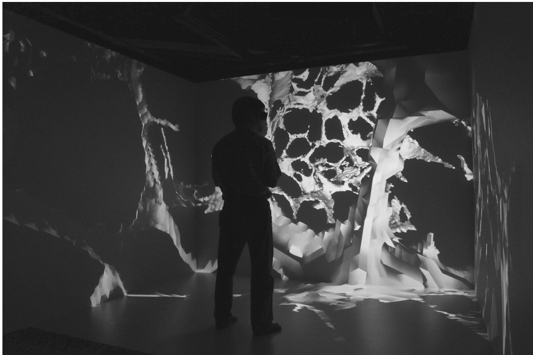
Figure 3. Data projected in the 3-D visualization cave in the Fossett Laboratory for Virtual Planetary Exploration at Washington University in Saint Louis. The visualization cave projects data onto three walls and the floor. Users, wearing 3-D glasses, are able to ‘fly’ into the sample and readily view objects from several orientations that might be obscured by other microstructural features.
